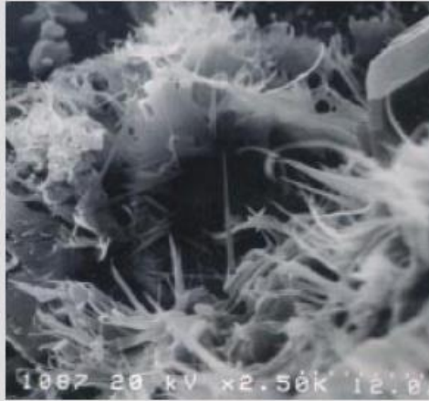
Fig. 14. Delicate wisps of "hairy" illite project into a pore. Note that the fibers not only form a highly rugose surface within the pore, but the fibers could break and migrate under extreme fluid pressures (x2500) (image courtesy of Westport Technology Center)
