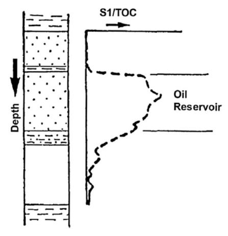
FIGURE 5.5 An example of using Rock-Eval S1 data to indicate the presence of an oil-bearing reservoir. *Modified after Dow, W.G., Talukdar, S.C., January* 1991. *Petroleum geochemistry in oil production*. Houston Geological Society Bulletin 33, 44–52.
