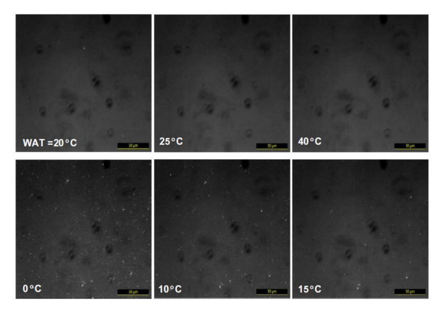
Fig. 5. Microscopic images of oil 2 at different temperatures (WAT = 20  $^{\circ}$ C).
