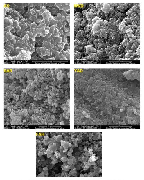
Fig. 10. SEM Images of Wax Particles of different oil samples isolated by the IP 143 method of crude oil.
