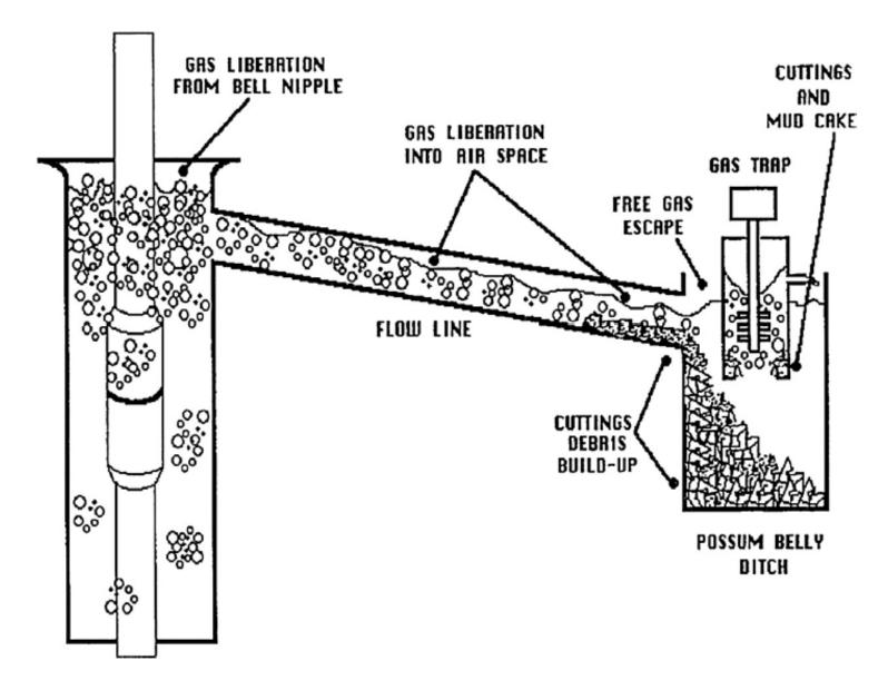
FIGURE 5.1 A schematic of the return mud flow on a drilling rig showing the location of the gas trap. Whittaker, A., 1991. Mud Logging Handbook. Prentice-Hall, Englewood Cliffs, NJ. 531 p.
