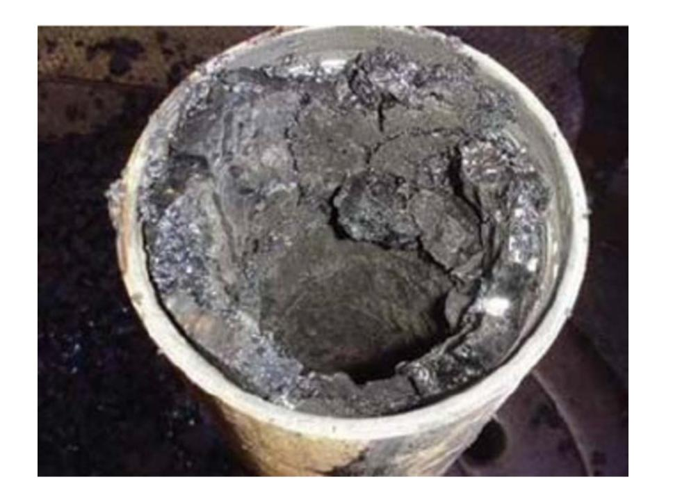
• High-molecular weight waxes (>C40) in crude oils can cause problems during production. These waxes are held in solution in the crude oil in the subsurface. As the oil is produced and leaves the reservoir, the temperature of the oil can decrease causing the high-molecular weight waxes to drop out of solution. This can result in wax deposition in the near borehole environment, the production lines to the surface, the flow lines from the wellhead, surface storage, and pipelines.
