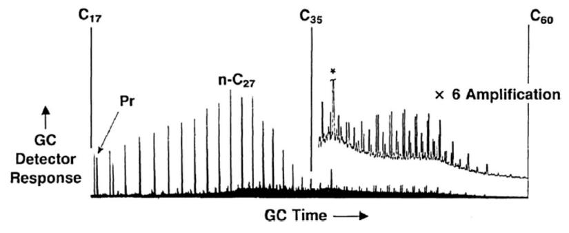
FIGURE 5.7 An example of a high-temperature gas chromatographic analysis for >C<sub>40</sub> waxes in a crude oil. GC, Gas chromatography. From Carlson, R.M.K., Teerman, S.C., Moldowan, J.M., Jacobson, S.R., Chan, E.I., Dorrough, K.S., Seetoo, W.C., Mertani, B., 1993. High temperature gas chromatography or high wax oils. In: Indonesian Petroleum Association, 22nd Annual Convention Proceeding, pp. 483–507.
