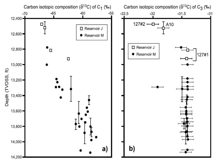
Figure 11. Carbon isotopic composition ( $\delta^{13}$ C) of C<sub>1</sub> (a) and C<sub>3</sub> (b) in fluids from the Horn Mountain field. These data include measurements from MDT, IsoTube, and separator samples. Error bars for most isotope measurements equal to 0.2% and are smaller than the size of symbols for C<sub>1</sub> (a). Error bars for depth are shown only for separator samples and correspond to the perforated intervals in producing wells.
