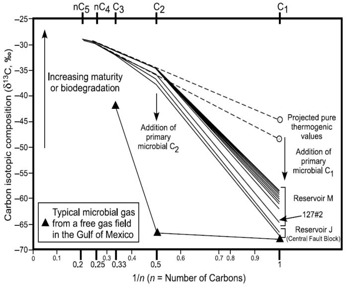
Figure 12. Carbon isotopic composition ( $\delta^{13}$ C) of C<sub>1</sub> - C<sub>5</sub> gases in the Horn Mountain field displayed on the natural gas plot (Chung et al., 1988). Dashed lines show extrapolation of carbon isotope values of  $C_2 - C_5$ gases to obtain the  $\delta^{13}$ C of pure thermogenic C<sub>1</sub> in gases (range from -48 to -45%). Precision and accuracy of isotope measurements are ±0.1%, which approximately corresponds to the thickness of lines.
