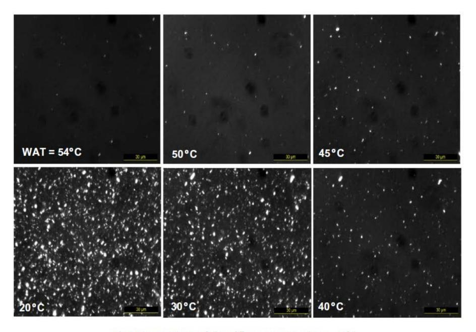
Fig. 6. Microscopic images of oil 3 at different temperatures (WAT = 54  $^{\circ}$ C).
