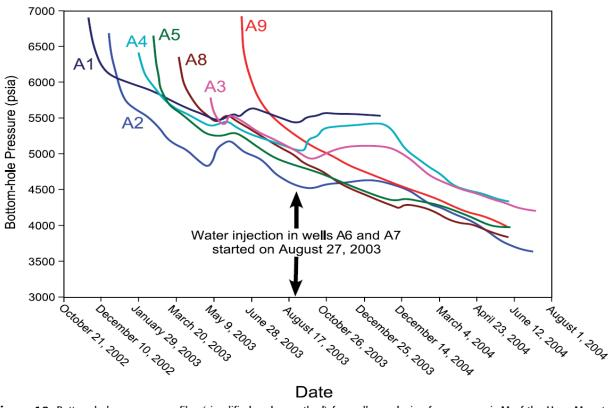
**Figure 18.** Bottom-hole pressure profiles (simplified and smoothed) for wells producing from reservoir M of the Horn Mountain field. Note how pressure increased in wells A1–A4 after water injection started, but no significant pressure increase was observed in wells A5, A8, and A9.
