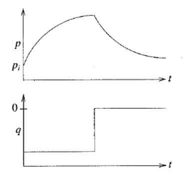
As with injection test, falloff test, interpretation is more difficult if the injected fluid is different from the original reservoir fluid.
