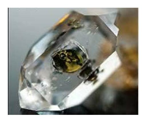
Fluid inclusions are imperfections in minerals that trap small quantities of oil, gas, and water. Primary inclusions form during initial mineral growth within intracrystalline microcavities, while secondary inclusions form during cementation and occur in intergranular pore space or in microfractures. Many minerals may contain fluid inclusions, but the most common in sedimentary basins are carbonates, silicates (quartz and feldspar), and evaporites (halite, anhydrite, and fluorite). Inclusion
