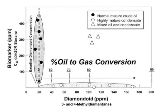
Because diamondoids are concentrated rather than created during cracking, the oil-to-gas cracking or diamondoid cracking ratio for a highly mature oil in the reservoir can be estimated from the increase in diamondoid concentration above the baseline concentrations in low-maturity oils. We use the simple formula:
