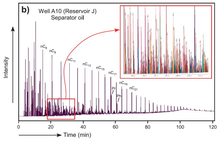
**Figure 5.** Typical WOGC of production oils from reservoir M (a) and J (b). Inserts show peaks in the  $n-C_{8.5}-n-C_{11.5}$  range (outputs from ReserView software; the same peaks in a and b have the same colors) used for WOGC fingerprinting.
