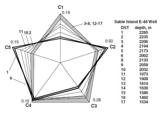
Figure 7.26. Halpern C<sub>7</sub> oil correlation star diagram for drill stem test (DST) samples from the Sable Island E-48 well, Scotian Shelf, Canada. The numbers at the end of each axis are endpoints for individual ratios. Two end-member oil groups are apparent. One group includes DST from depths of 1460–1908 m and 2133–2206 m (DST 12–17, 3–8). The other end member consists of DST 1 and 9. DST 2, 10, and 11 are mixtures of the two end-member fluids.
