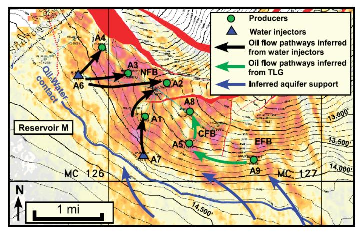
**Figure 21.** Fluid-migration pathways during production of reservoir M as inferred from the analysis of pressure response to water injection and from time-lapse geochemistry.
