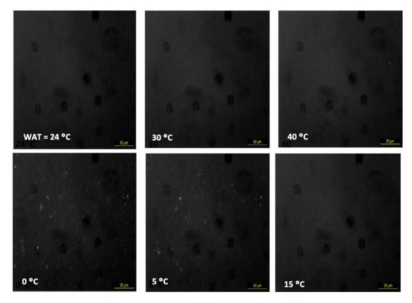
Fig. 4. Microscopic images of oil 1 at different temperatures (WAT =  $24 \, ^{\circ}$ C).
