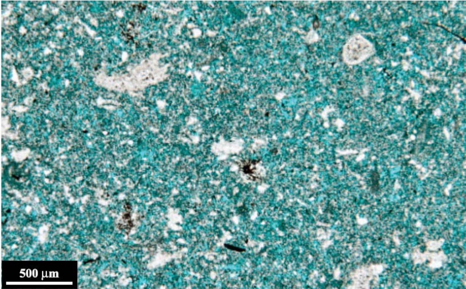
Mesoporosity (20–60  $\mu\text{m}$  pore diameter) with uniform porosity distribution,  $f = 19.3\%$ ,  $k = 4.93 \text{ md}$ ;
