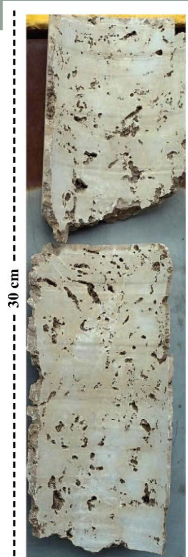
Core slabs showing vuggy porosity. Plug-derived porosities and permeabilities are strongly dependent on the location of core plugs because of the large vug sizes.
