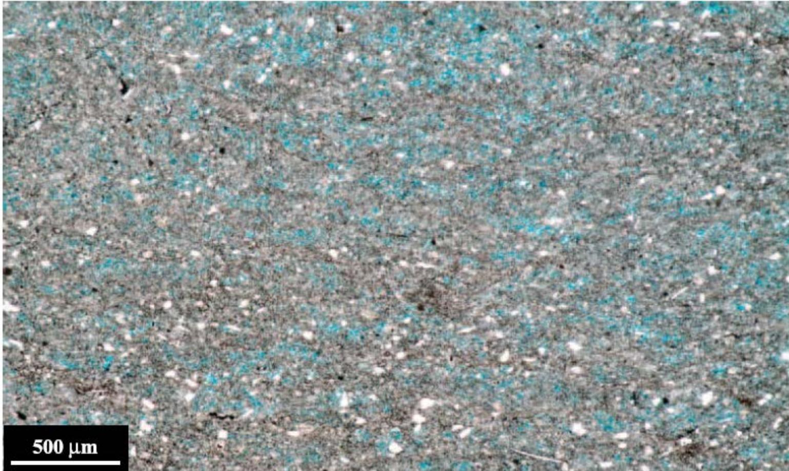
microporosity (10–20 mm pore diameter) with uniform porosity distribution,  $f = 18.1\%$ ,  $k = 0.476$  md;
