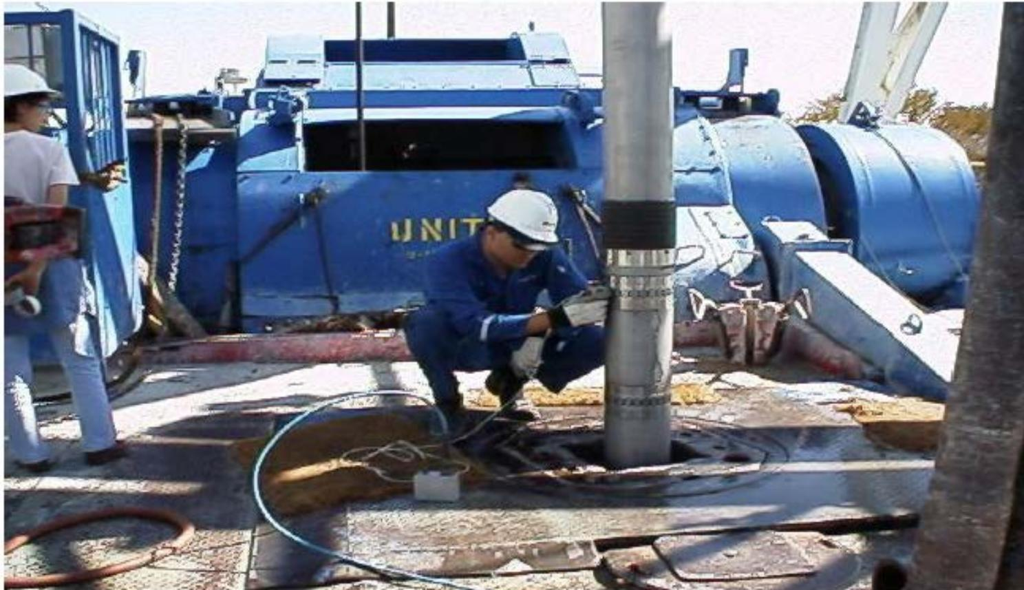
Synchronization check of the clock and the entire system during a shallow hole test prior to running in the hole.
