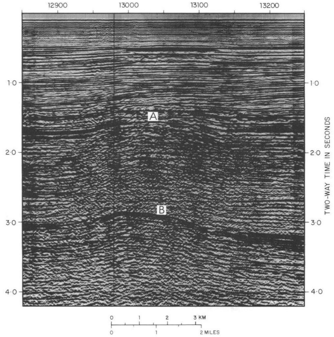
**FIGURE 4.49** Bright spot in a shallow-gas sand above a deeper salt structure. Courtesy Merlin Profilers Ltd.
