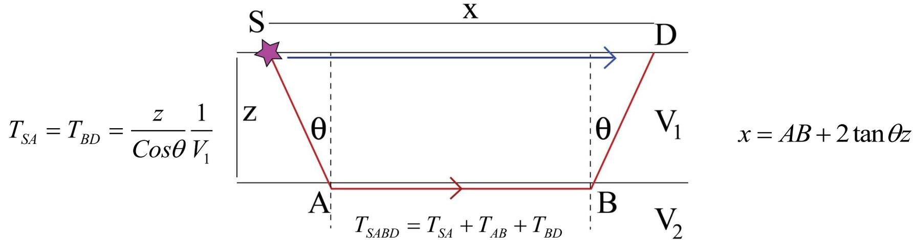
$$T_{SABD} = \frac{2z}{\cos\theta} \frac{1}{V_1} + \frac{x - 2 \tan\theta z}{V_2} = \frac{x}{V_2} + 2z \left( \frac{1}{\cos\theta V_1} - \frac{\tan\theta}{V_2} \right) = \frac{x}{V_2} + \frac{2z}{\cos\theta V_1} \left( 1 - \frac{V_1 \sin\theta}{V_2} \right) = \frac{x}{V_2} + \frac{2z}{\cos\theta V_1} (1 - \sin^2\theta)$$
