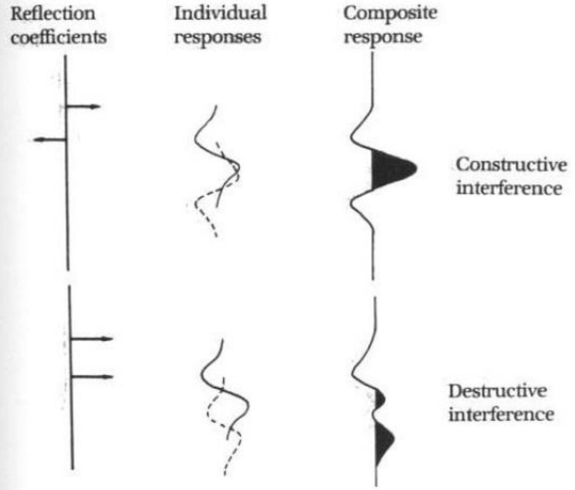
**FIGURE 2.10** *Constructive and destructive interference affecting a minimum-phase normal-polarity wavelet.*
