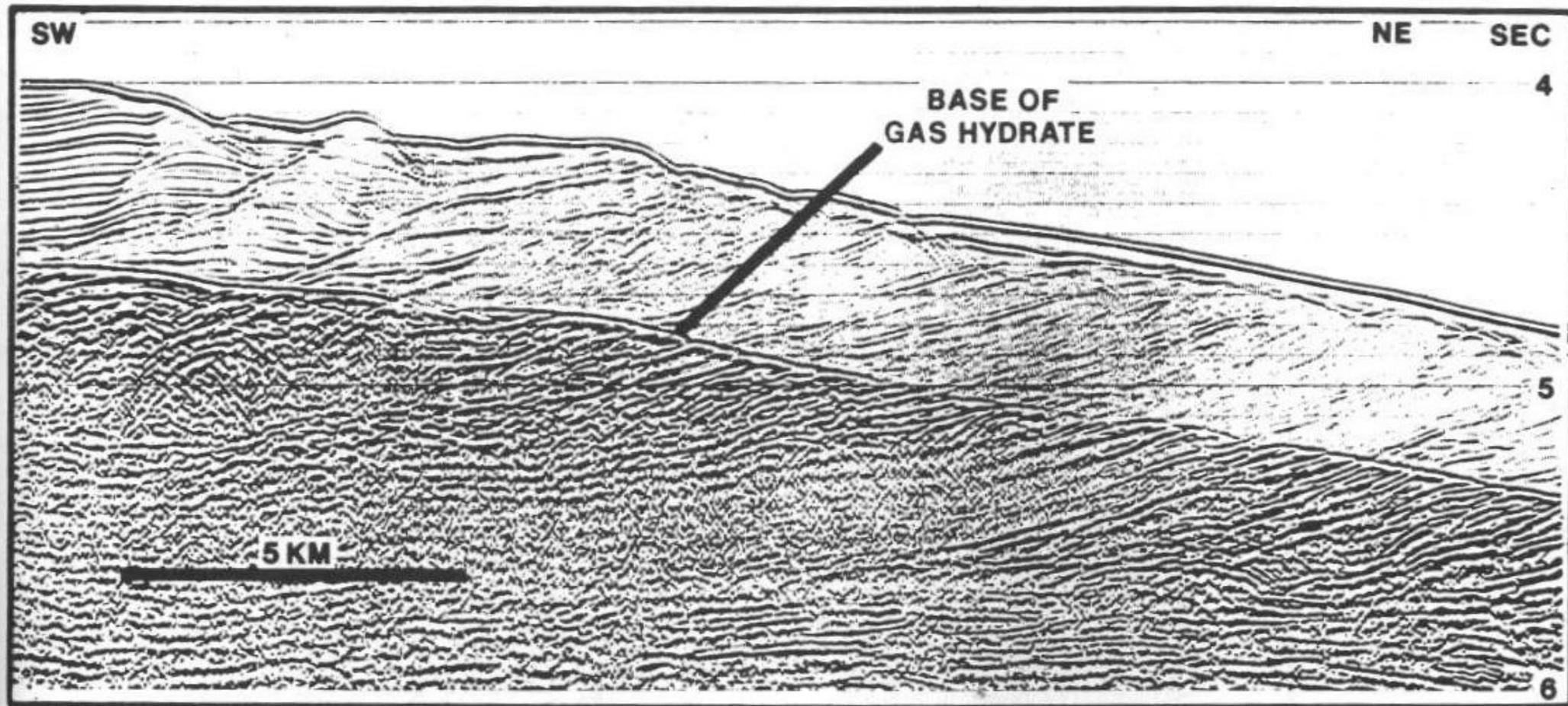
**FIGURE 4.55** Seismic section from the eastern flank of the Blake Outer Ridge. The reflection at the base of the gas hydrate follows the sea-floor bathymetry and crosscuts dipping reflections. The lower amplitude of reflections above the gas hydrate may be the result of reduced acoustic-impedance contrasts in the presence of the gas hydrate. Reprinted by permission of the AAPG from Shipley et al., 1979.
