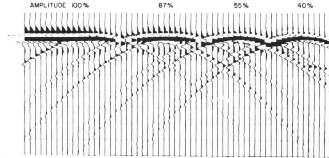
(b) Wave-theory model response for sandstone bodies of varying lateral extents illustrating significance of Fresnel zone size.
