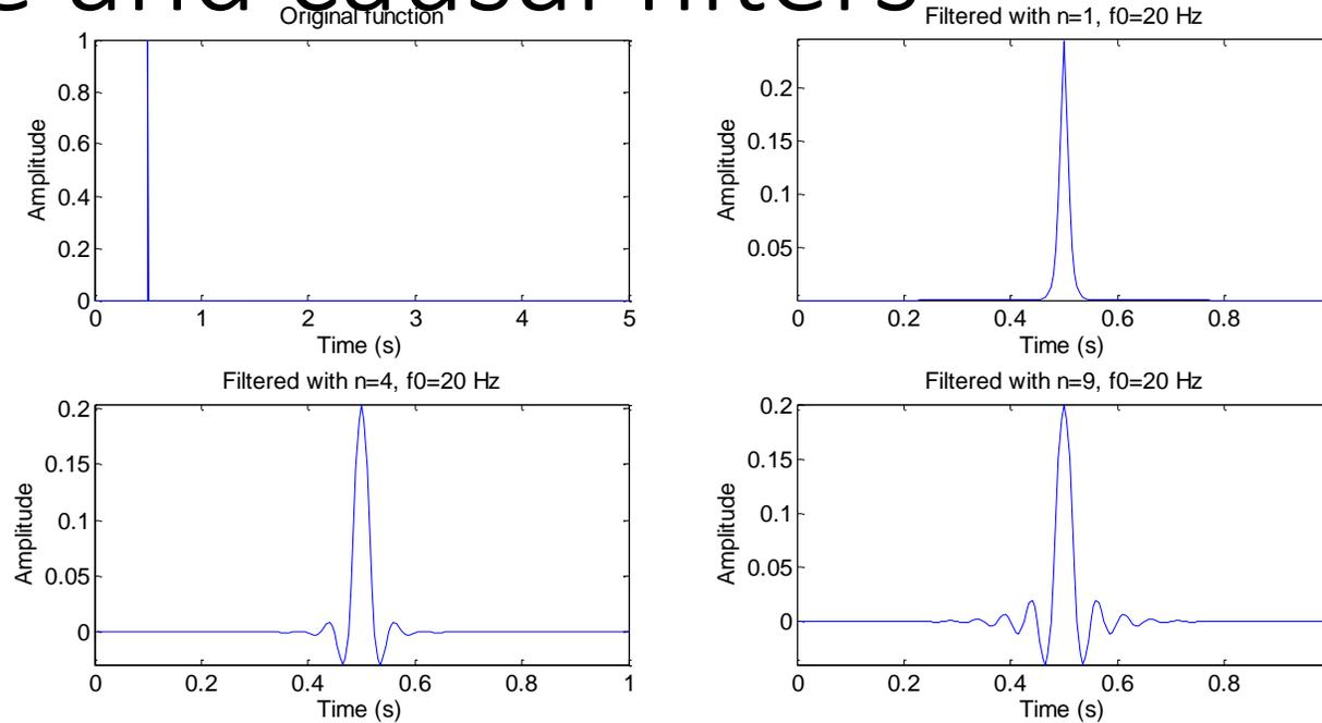
When the phase of a filter is set to zero (and simply the amplitude spectrum is inverted) we obtain a **zero-phase filter**. It means a peak will not be shifted.
