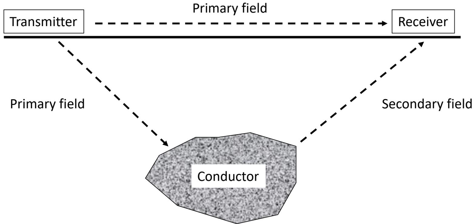
Electromagnetic anomaly = Primary Field – Secondary Field
