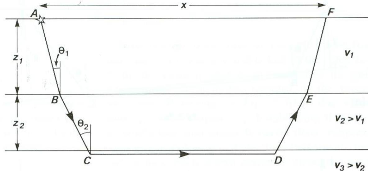
*ABCDEF* is the refracted ray path through the bottom layer of a three layer model. The travel time curve for the direct and two head waves are shown above.
