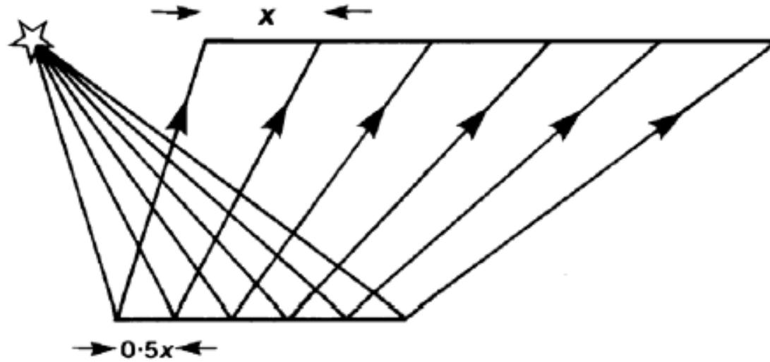
Horizontal Resolution = half the detector spacing
