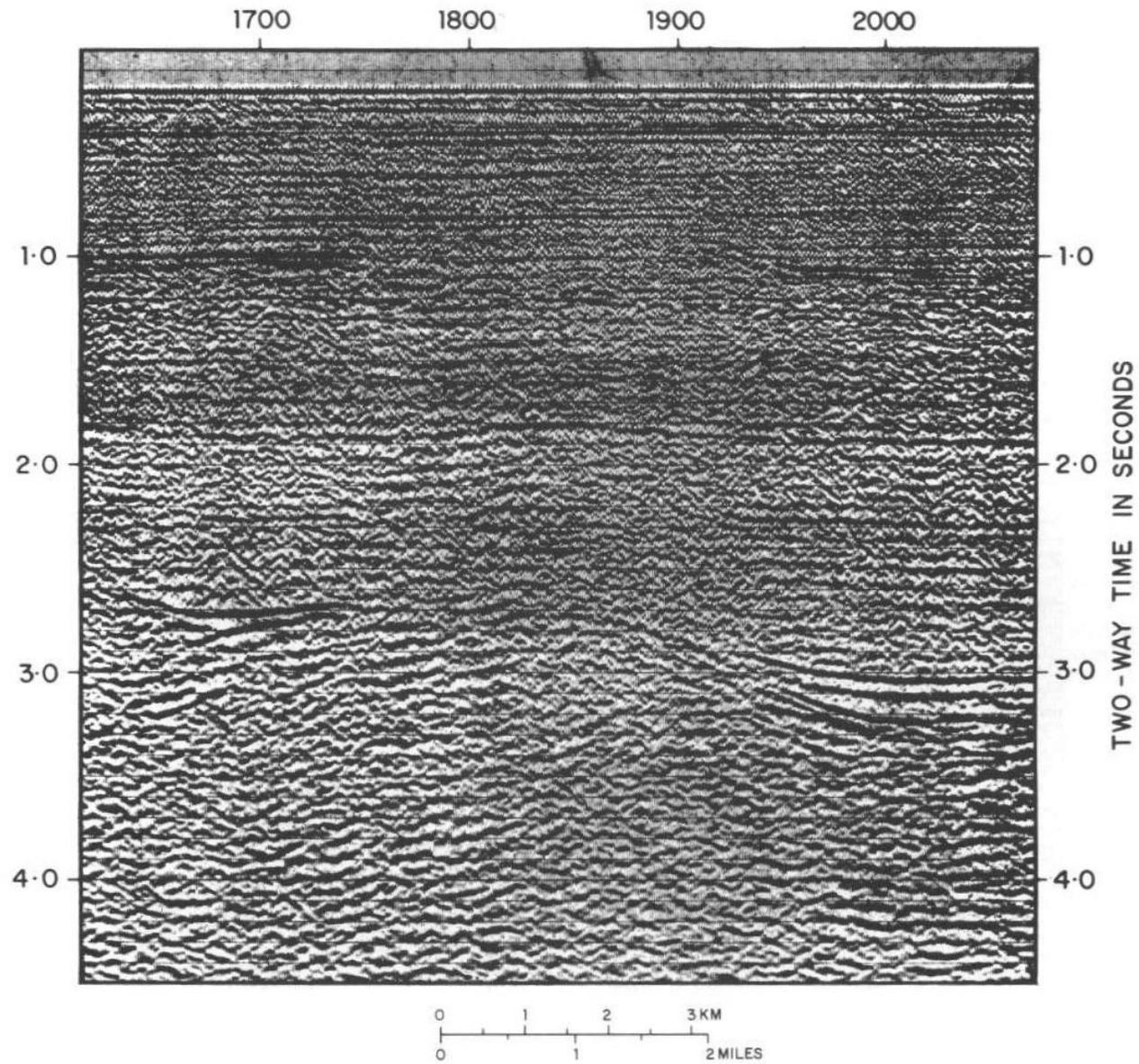
**FIGURE 4.52** Gas-chimney effect above the gas-bearing 34/10 alpha structure, offshore Norway. Courtesy Norsk Hydro.
