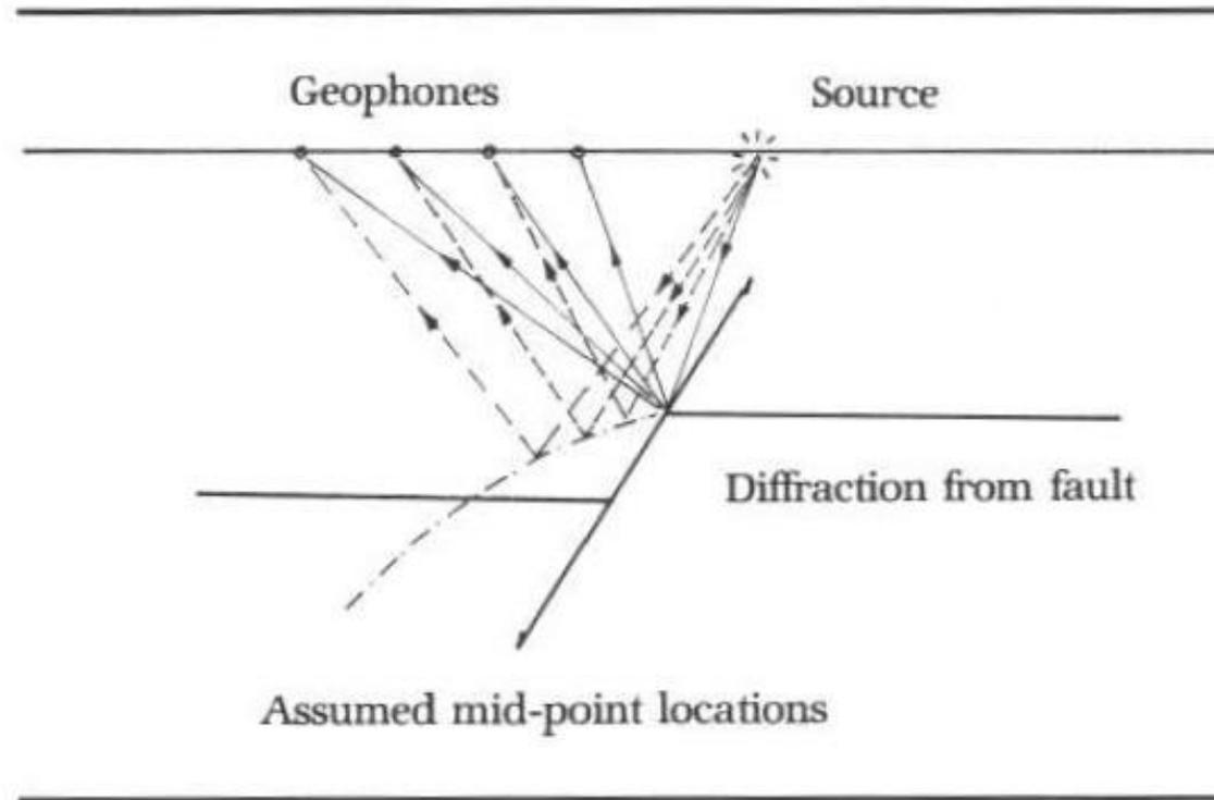
**FIGURE 3.16** Sketch showing a diffraction from a fault. The hyperbolic form of diffractions arises from the assumption made by the CMP method that reflections arise from mid-point locations between the source and geophone.
