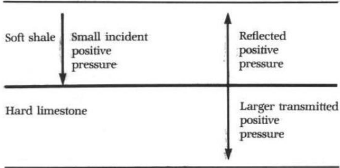
**FIGURE 2.4** Continuity of particle pressure at a soft-to-hard interface. The arrows indicate the raypath direction. Reprinted by permission of IHRDC Press from Robinson, 1983, fig. 3.16, p. 145.
