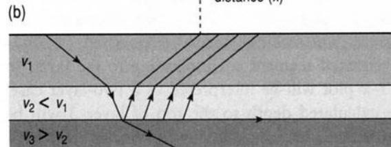
A **low velocity layer** that does not generate a head wave
