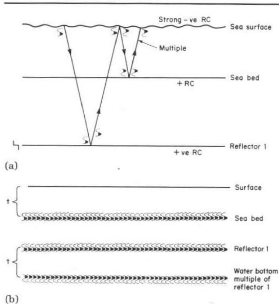
**FIGURE 3.12** Water-bottom multiples. (a) Geological model. (b) Seismic expression (SEG normal polarity). The strong negative reflection coefficient of the air/water interface causes a polarity reversal of the downgoing multiple reflection. The positive sea-bed reflection coefficient does not affect the reflection polarity; therefore, the recorded multiple reflection is opposite in polarity to that of the primary reflection.
