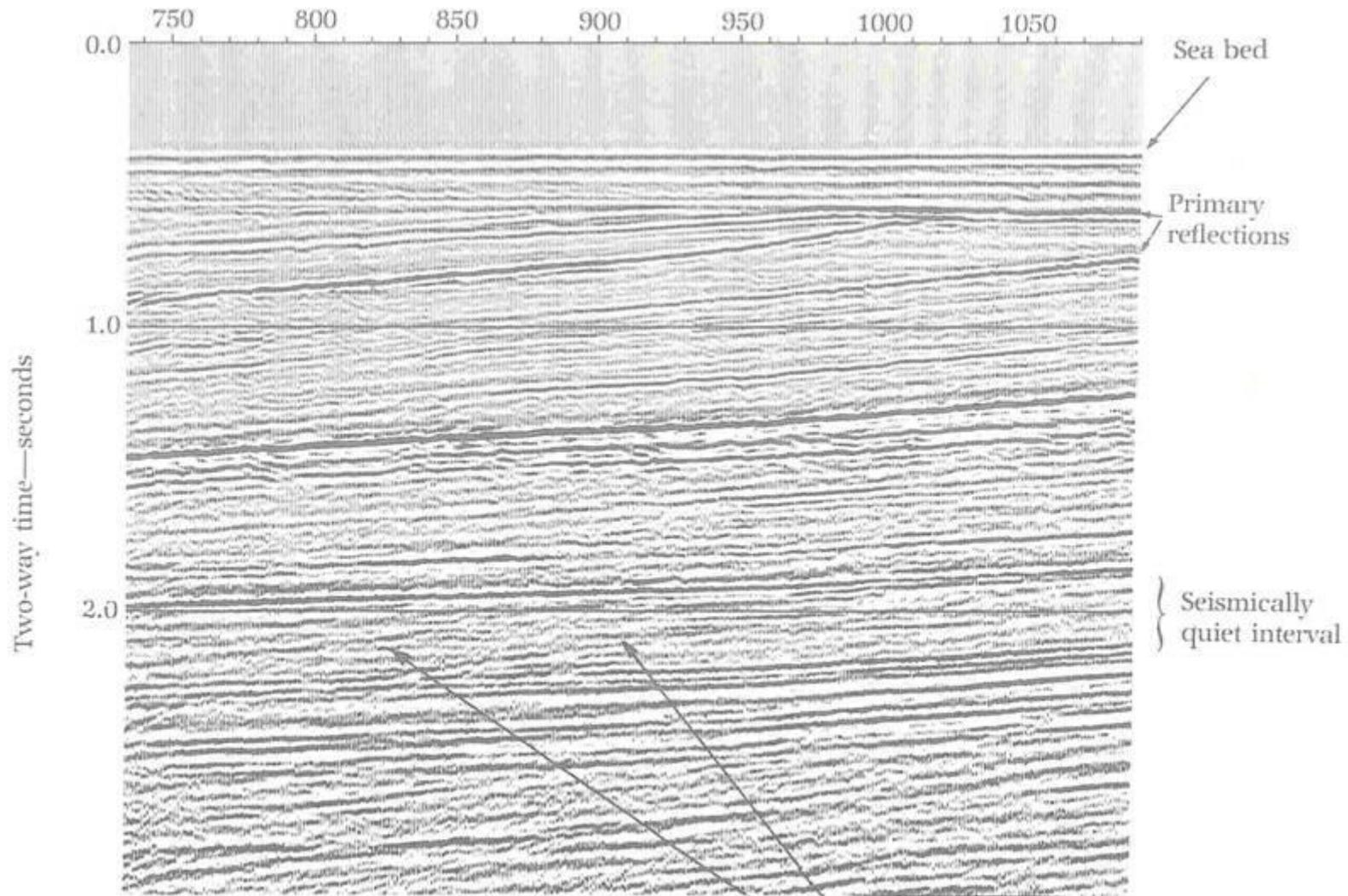
Dipping reflections in a seismically quiet interval—
