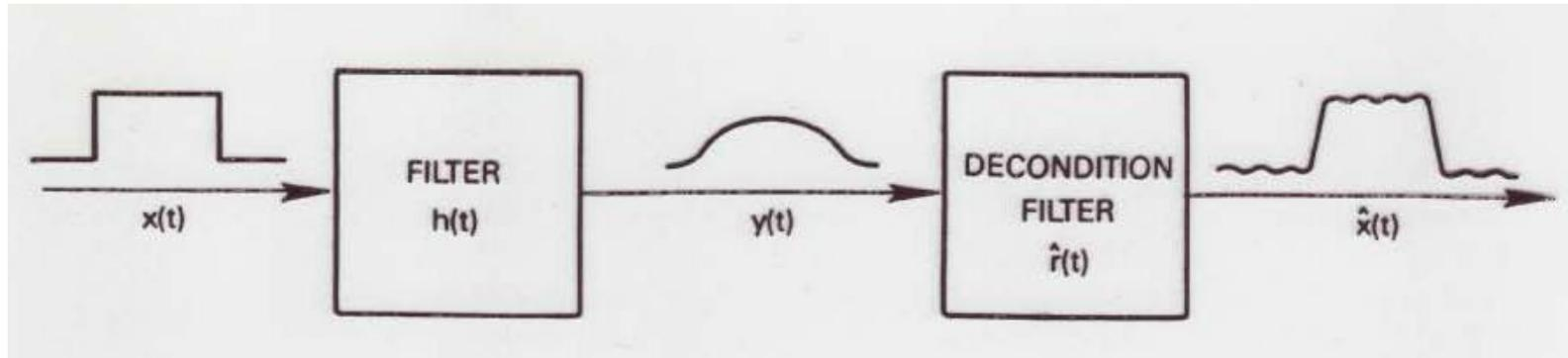
For this reason, a further process called *deconvolution* must be performed to recover the input signal  $x(t)$ . Unfortunately, the input signal  $x(t)$  is never recovered *completely*. Thus, the signal recovered by the *decondition filter* is not *exactly* equal to  $x(t)$ . Nevertheless, if the deconvolution process is well done, the recovered signal can be used instead of the original signal  $x(t)$ , with a small error (Brigham, 1988).
