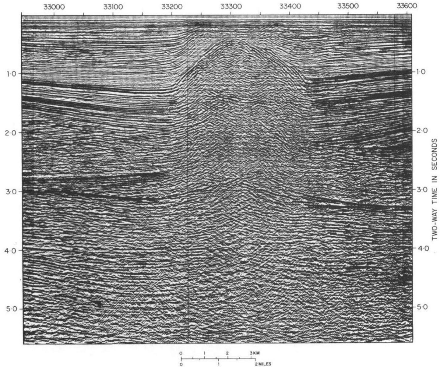
**FIGURE 3.33** *Seismic section across a salt diapir. Courtesy Merlin Profilers Ltd.*
