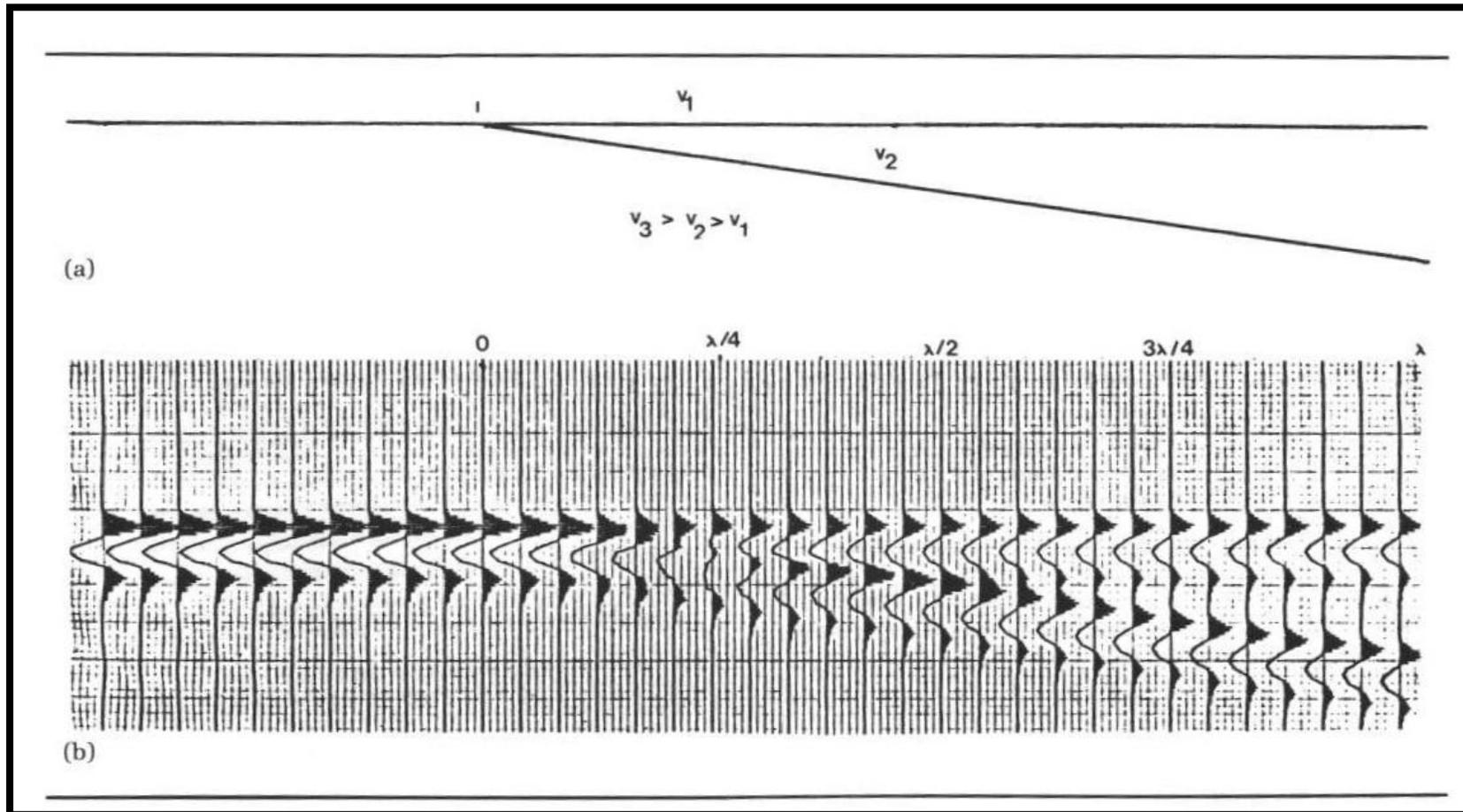
**FIGURE 2.16** Reflection from a wedge of acoustic impedance intermediate in magnitude between that of the over- and underlying units. The thickness of the wedge is indicated as a fraction of the dominant wavelength. Note that there is still a reflection beyond the limit of the wedge due to the contrast in acoustic impedance between the over- and underlying layers. (a) Model. (b) Seismic section. Reprinted by permission of the EAEG from Sheriff, 1975, fig. 6.9, p. 128.
