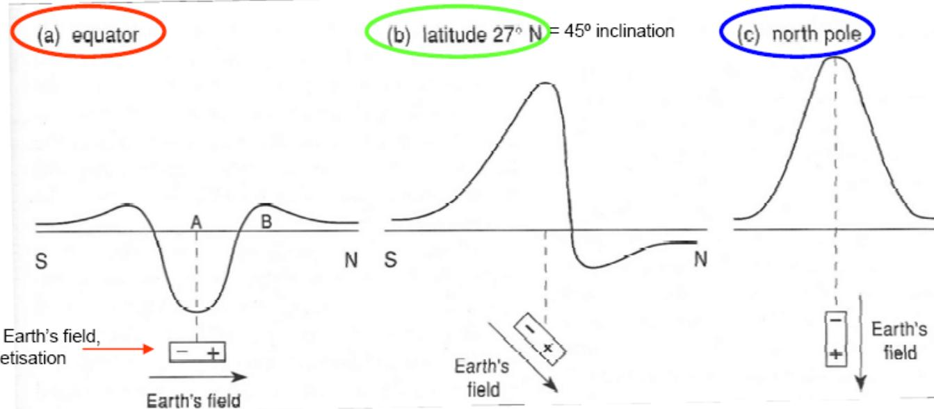
dipole aligned with the Earth's field, i.e. only induced magnetisation
