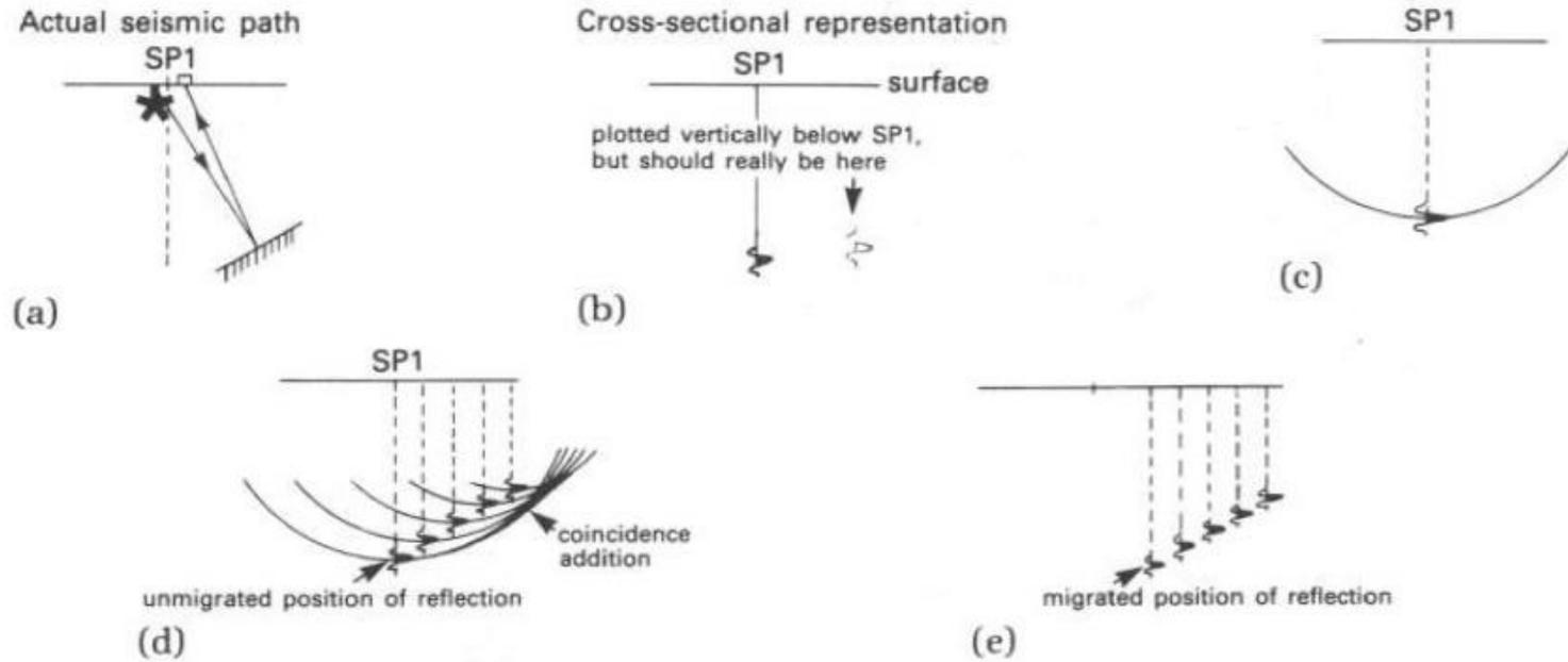
**FIGURE 3.23** A simple view of the process of migration. See text discussion. Reprinted by permission of IHRDC Press from Anstey, 1980a, fig. 4, p. 8.
