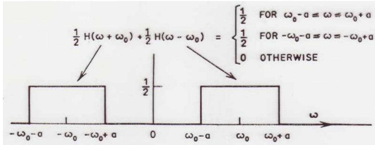
This filter is a *band-pass* filter. The effects of this kind of filter can be observed by using of the program [SPECTRUM](#).
