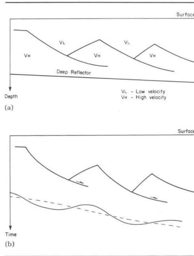
**FIGURE 3.31** Velocity anomalies beneath detached listric-normal faults. (a) Geological model showing a set of detached listric-normal faults and associated tilted fault blocks. The faults are underlain by a planar dipping reflector. (b) Seismic expression showing velocity pull-up beneath the tilted fault blocks and velocity push-down beneath the intervals of thick low-velocity infill. As a general rule, beware of deeper reflections that mimic the structure of shallower reflections.
