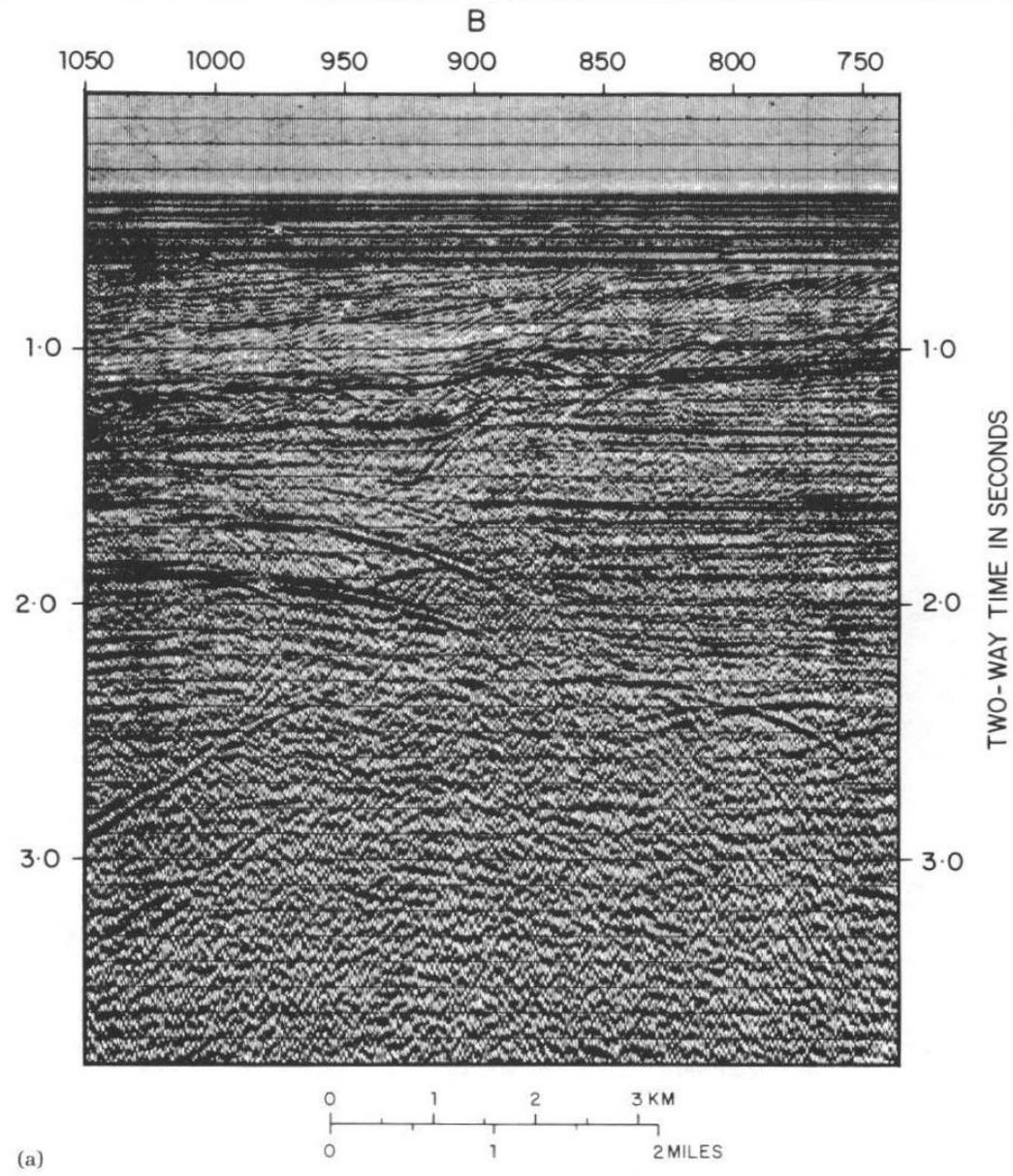
**FIGURE 3.28** Examples of stacked and migrated seismic sections. (a) Stacked section. (b) Migrated section. Courtesy Norsk Hydro.
