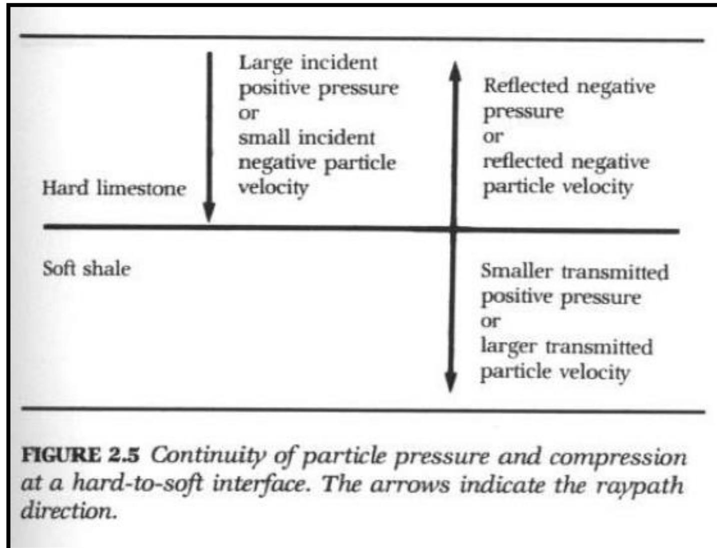
**FIGURE 2.5** Continuity of particle pressure and compression at a hard-to-soft interface. The arrows indicate the raypath direction.
