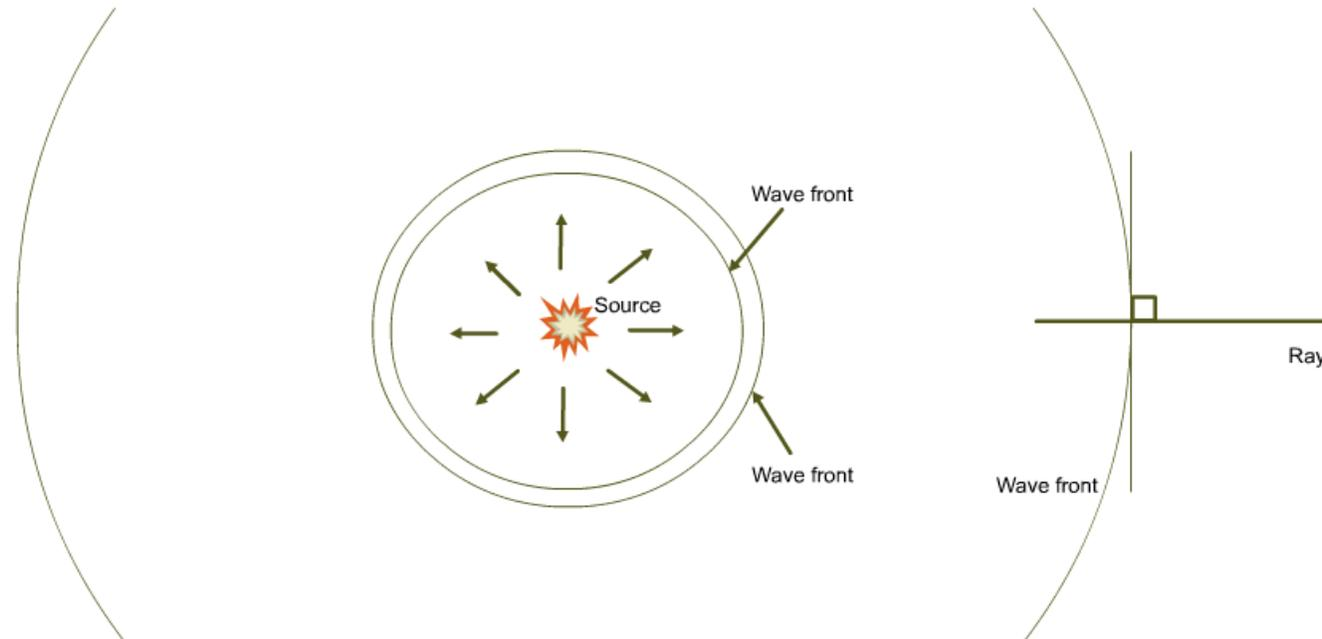
The seismic wave along one wave front has always the same phase. At large distance from the source the wave front is close to planar, and the wave is called a plane wave.
