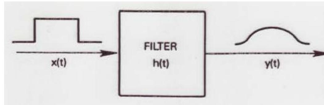
where  $h(t)$  is determined by the system properties. This general definition of a filter must be restricted to apply the spectral analysis, performed by the FFT. For it, the system given by  $h(t)$  must satisfy the fundamental properties listed below (bath, 1974).
