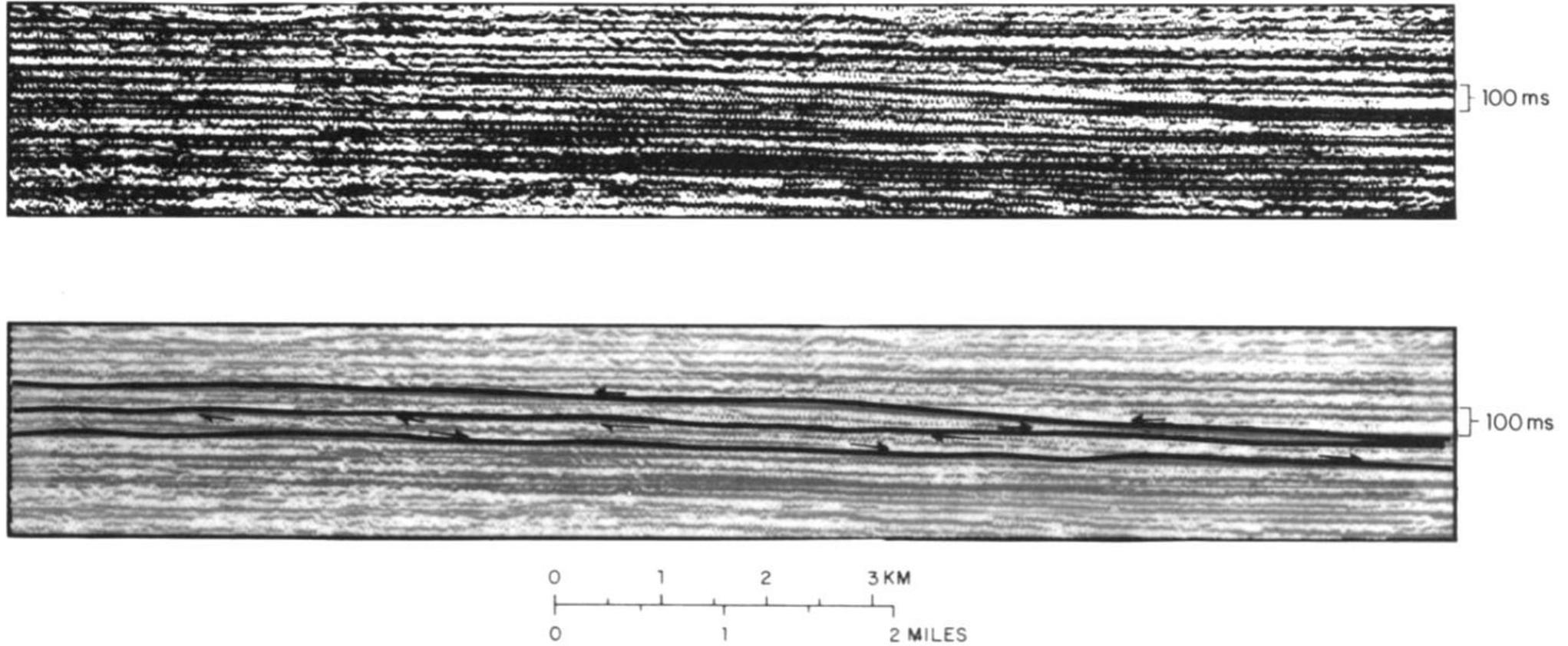
**FIGURE 4.31** Seismic section across a major shallow-marine clastic complex. The tapered profile is typical of clastic deposits. Courtesy Norsk Hydro.
