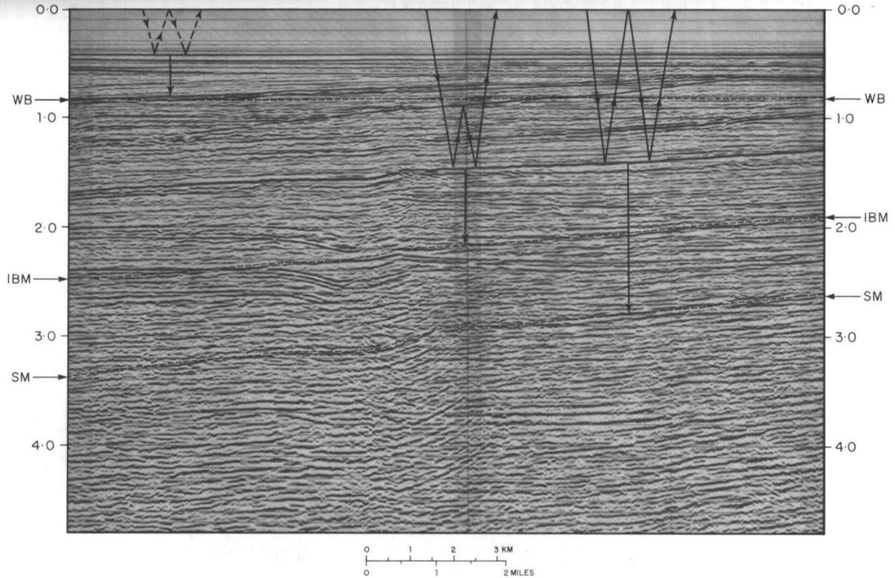
**FIGURE 3.10** A seismic section with a "good" set of multiples. SM, simple multiple; WB, water-bottom multiple; IBM, interbed multiple. Courtesy Société Nationale Elf Aquitaine.
