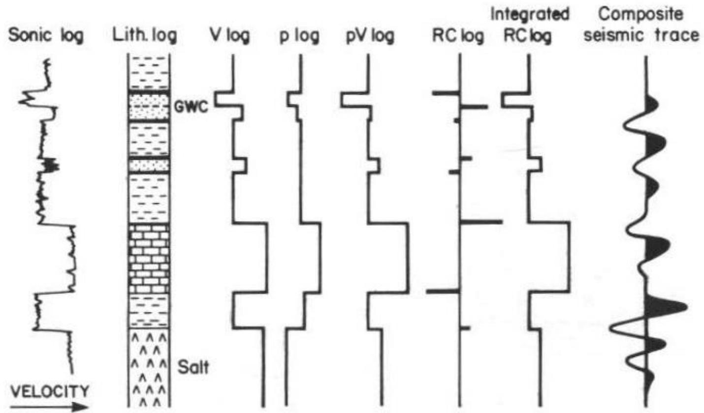
**FIGURE 2.9** Diagram showing the difference in resolution between a wireline sonic log and a seismic trace. After Anstey,
