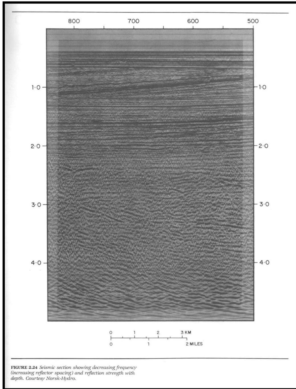
**FIGURE 2.24** Seismic section showing decreasing frequency (increasing reflector spacing) and reflection strength with depth. Courtesy Norsk-Hydro.
