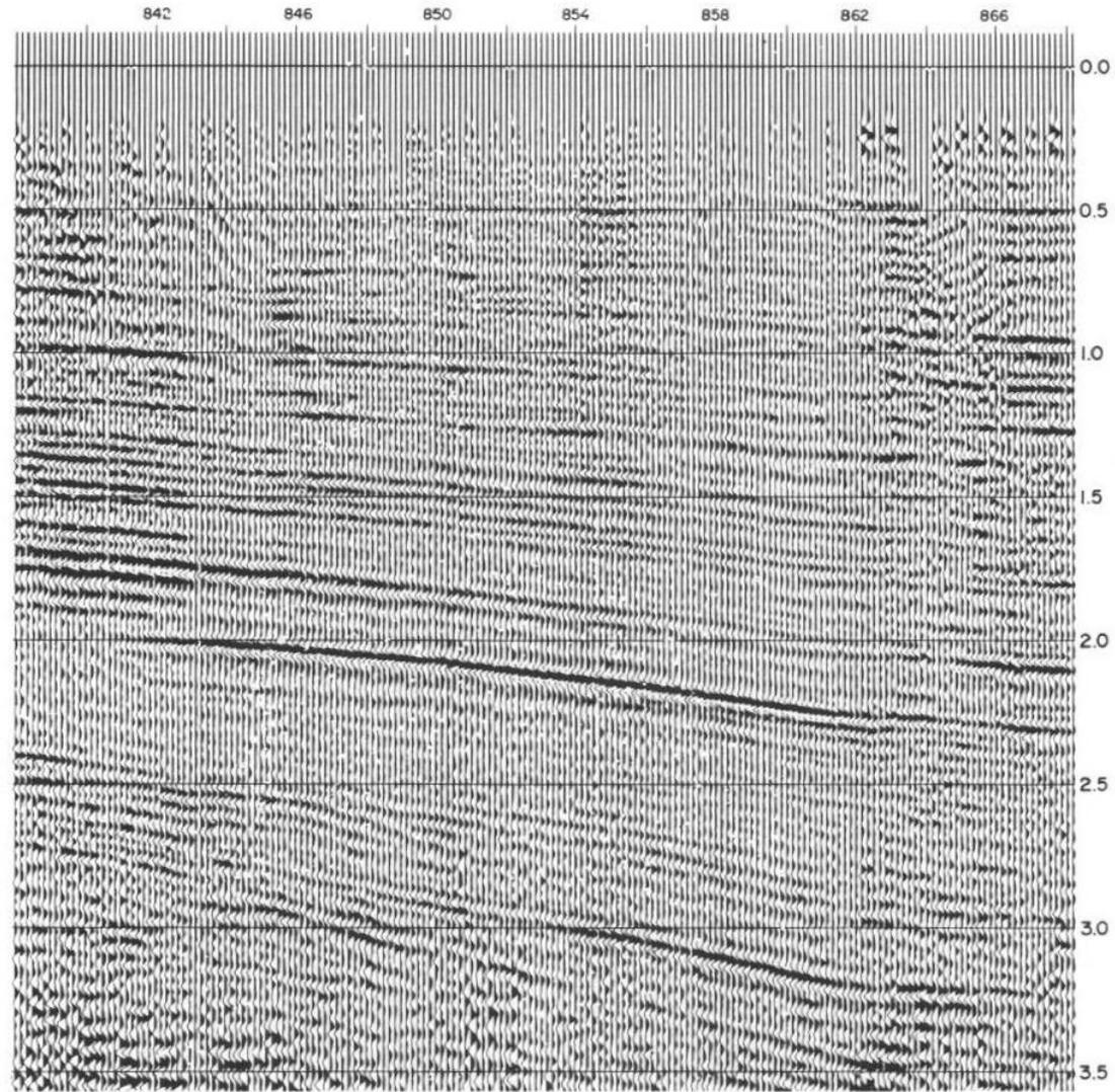
**FIGURE 4.53** Amplitude anomaly generated by a carbonate unit within a comparatively low-velocity sand/shale sequence. The bright spot is not related to hydrocarbons. Reprinted by permission of Teledyne Exploration Company from Barry and Shugart, 1973.
