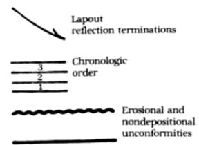
FIGURE 4.16 Seismic reflection configurations that define unconformities. Reprinted by permission of the AAPG from Brown and Fisher, 1980, fig. 46, p. 82.
