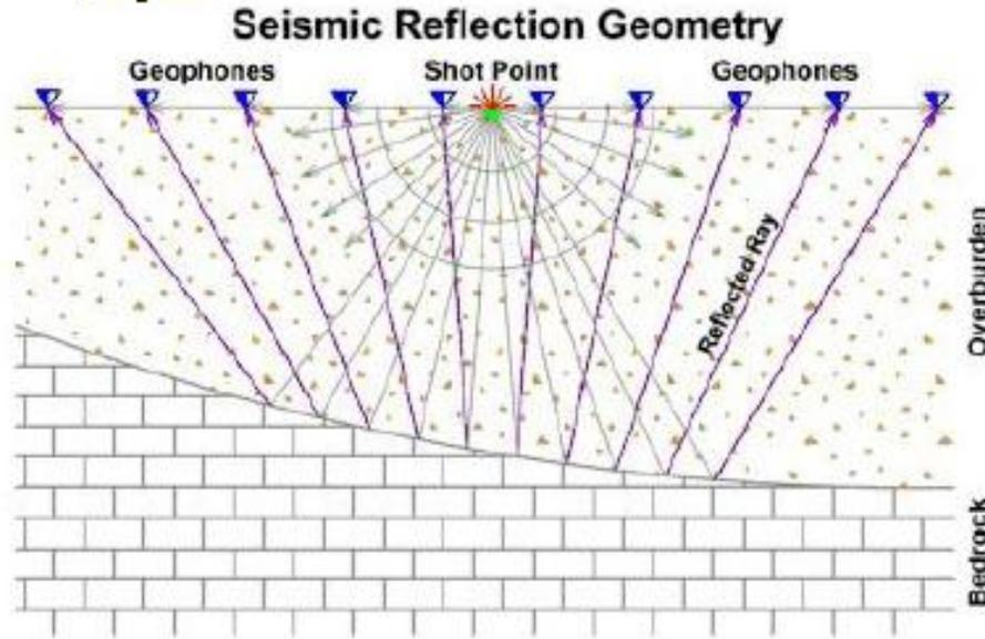
**Seismic Reflection** uses field equipment similar to seismic refraction, but field and data processing procedures are employed to maximize the energy reflected along near vertical ray paths by subsurface density contrasts.
