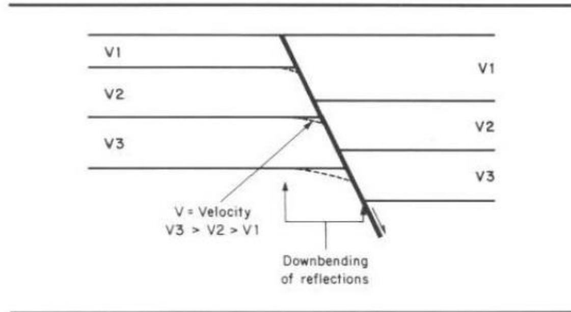
**FIGURE 3.30** *Downbending of reflections into a fault. This can occur when low-velocity material is faulted by a dipping fault. In the zone beneath the fault plane, downbending of reflections can occur due to the lower velocities (and, therefore, longer traveltimes) in lower-velocity downthrown rocks.*
