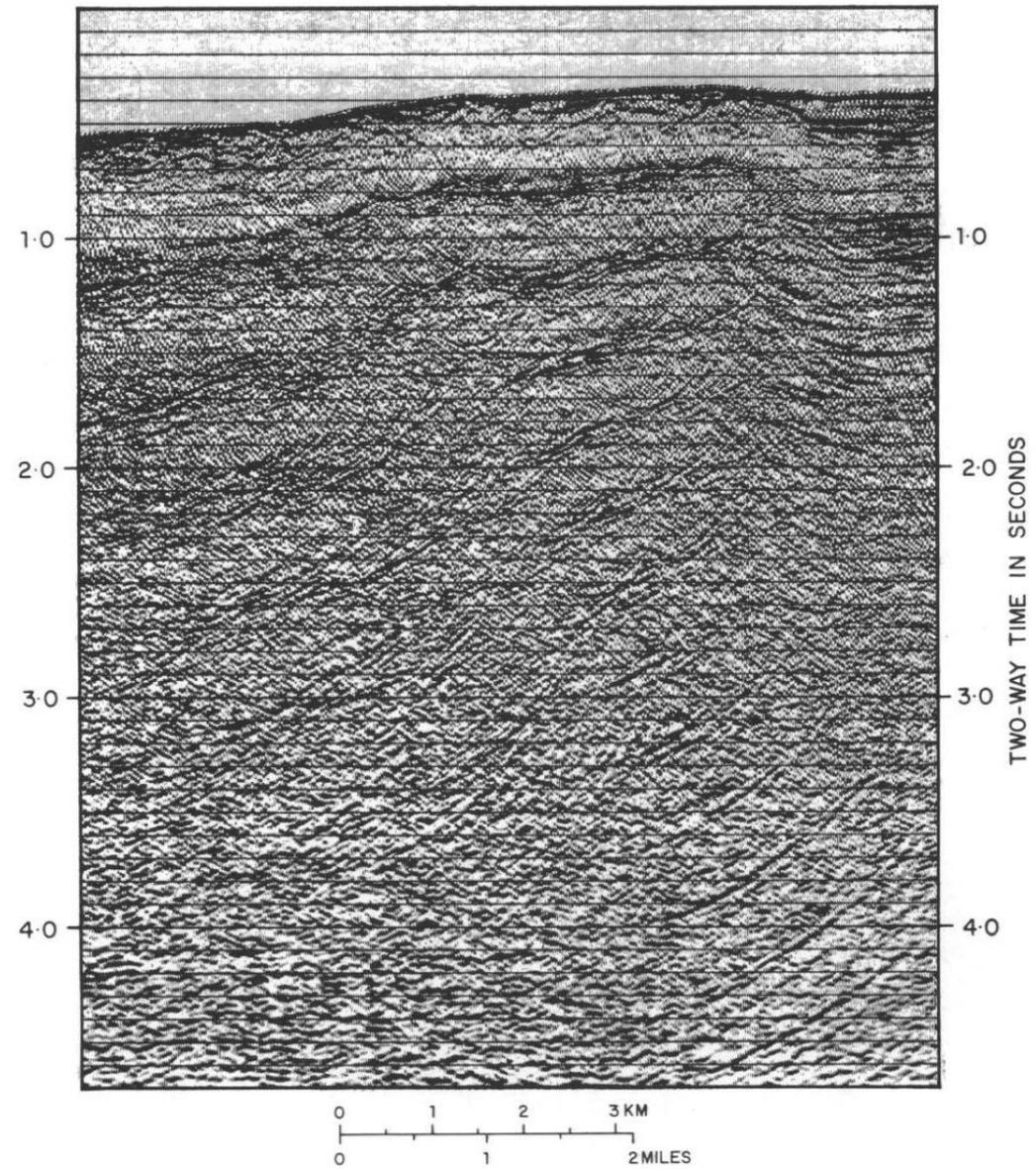
**FIGURE 3.11** Seismic section, with crystalline basement outcropping at the sea floor, showing water-bottom multiples. The water-bottom multiple is repeated 12 times. Note: The section has been migrated, and this has caused the dipping parts of the multiple to be moved in an updip direction. Courtesy Saga Petroleum.
