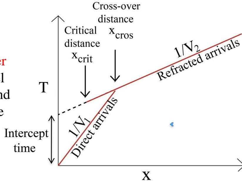
$$\frac{x_{cros}}{V_1} = \frac{x_{cros}}{V_2} + \frac{2z}{V_1 V_2} (V_2^2 - V_1^2)^{1/2}$$
