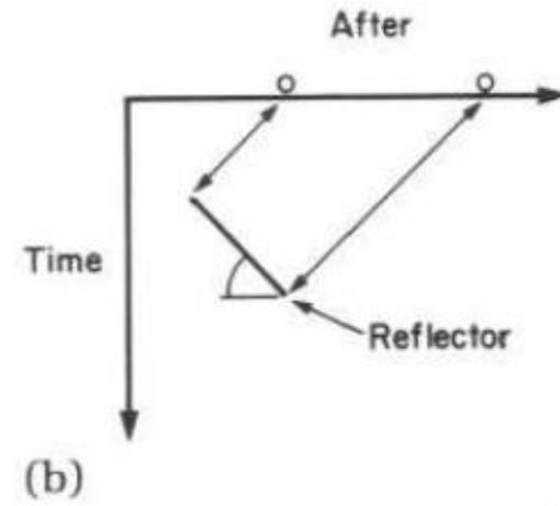
**FIGURE 3.22** *The effect of migration. (a) Before migration. (b) After migration. Migration increases reflection dip, moves the reflection updip, and shortens the reflection length.*
