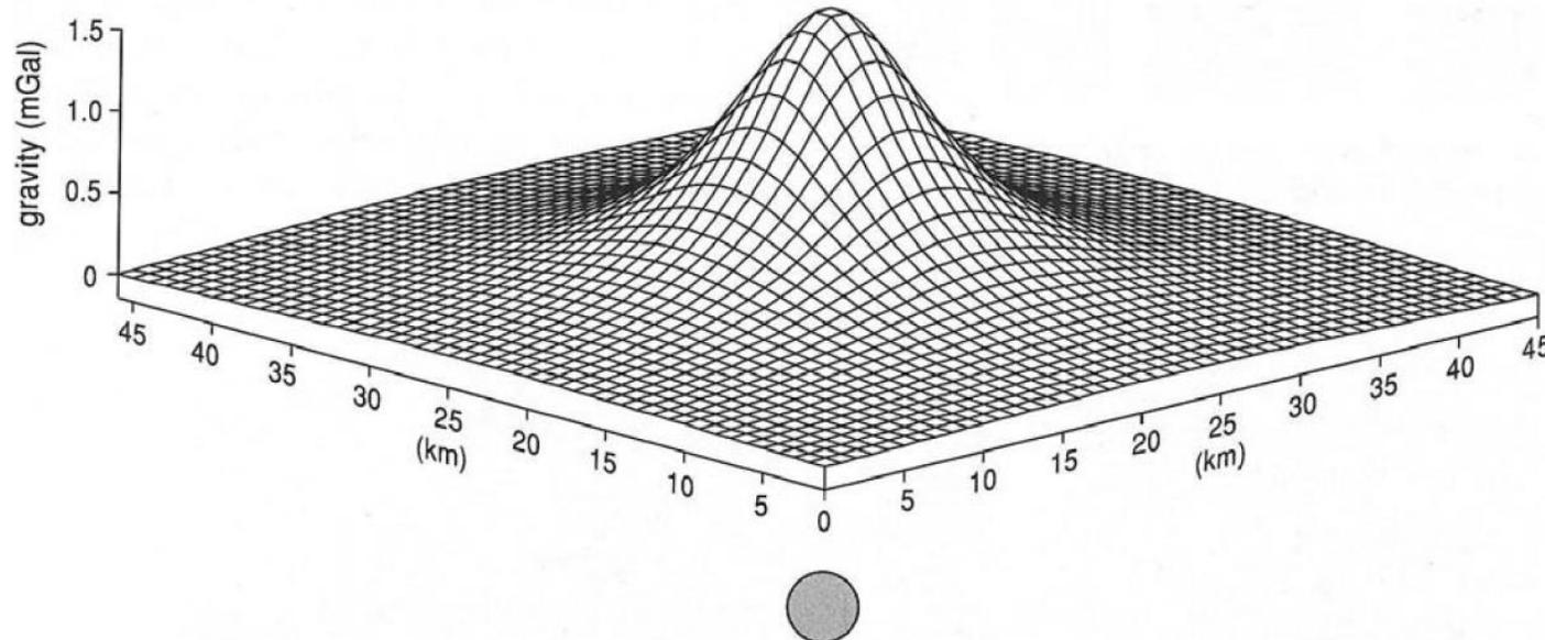
Gravity is a scalar: the combined pull has approx. The same direction as the Earth pull; we measure therefore only the size, or magnitude, of  $g$
