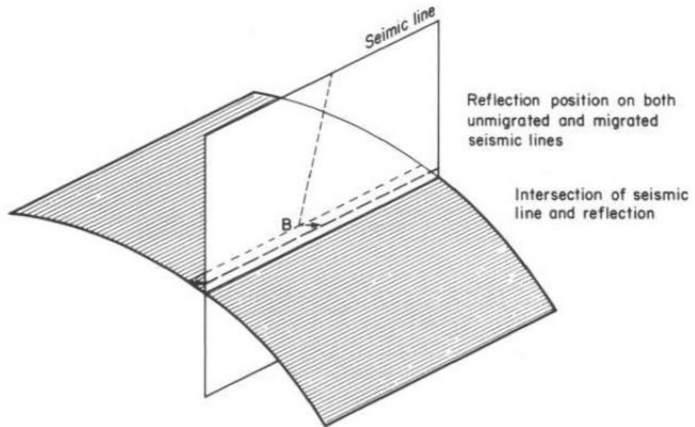
B - reflection originates updip from, and out of the plane of the seismic section
