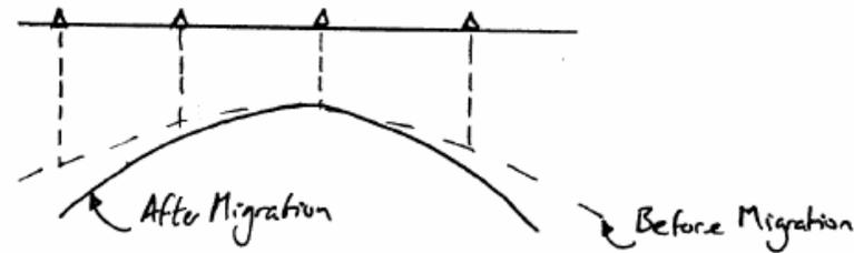
Reflections move upward and steeper during migration. Therefore anticlines look smaller in migrated sections.
