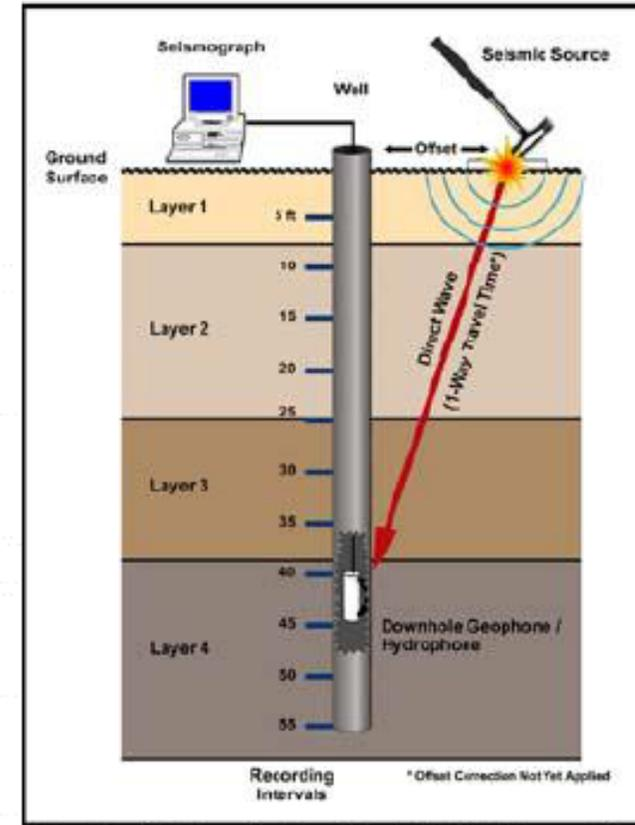
Vertical Seismic Profile (VSP) Schematic
