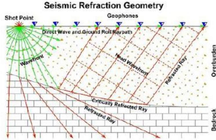
**Seismic Refraction** involves measuring the travel time of the component of seismic energy which travels down to the top of rock (or other distinct density contrast), is refracted along the top of rock, and returns to the surface.
