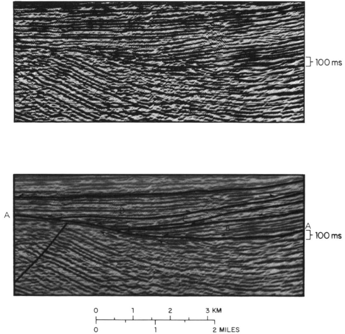
**FIGURE 4.26** Seismic example showing a subcrop sequence truncated beneath an unconformity A, which is downlapped by sequences B and C. Sequence C is overlapped from the left by sequence D. Courtesy Merlin Profilers Ltd.
