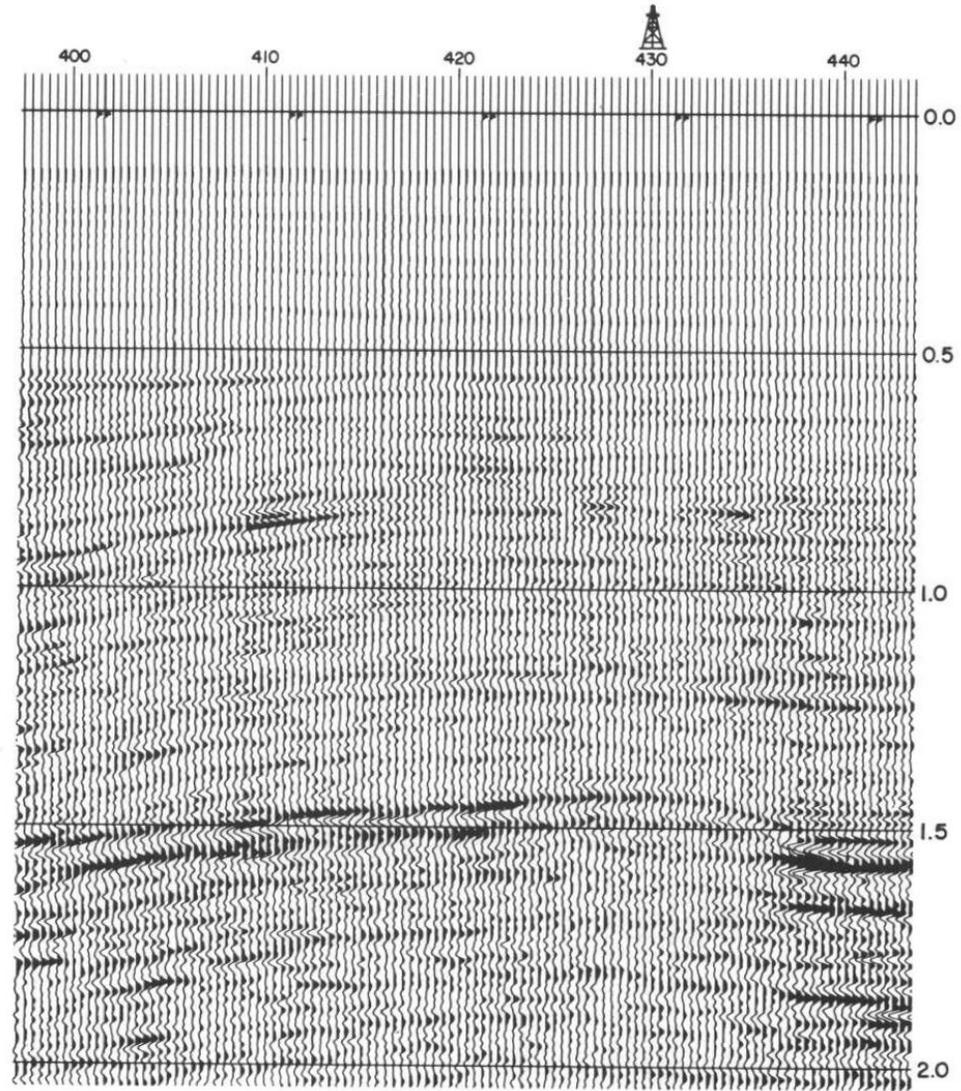
FIGURE 4.50 Dim spot associated with a gas-bearing porous carbonate overlain by interbedded sands and shales. Reprinted by permission of Teledyne Exploration Company from Barry and Shugart, 1973.
