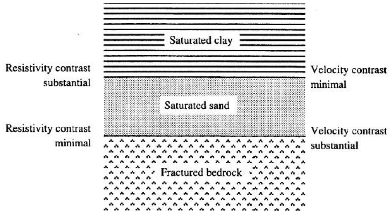
**Figure 1-1** Determining the thickness of a confined aquifer by using both seismic refraction and electrical resistivity.
