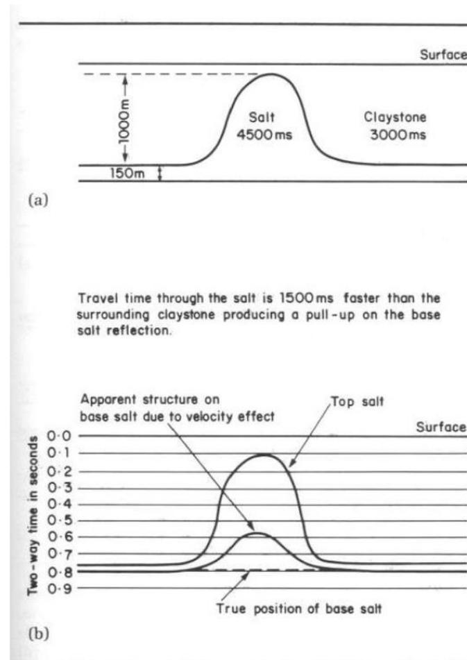
**FIGURE 3.34** Velocity anomaly beneath a salt diapir. (a) Geological model showing a salt diapir 1000 m high. (b) Seismic expression showing pull-up of 222 ms on the base salt reflector beneath the salt diapir.
