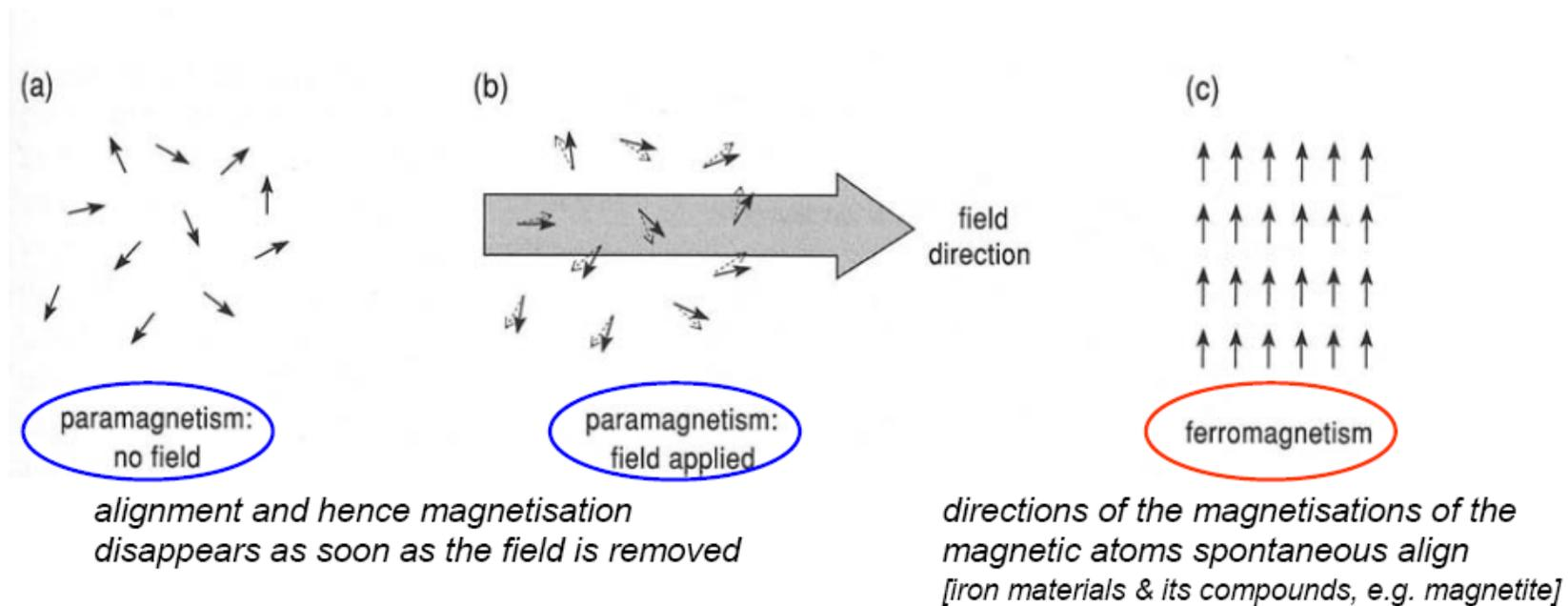
**Magnetic susceptibility ( $\chi$ ):** the ability of a rock to become temporarily magnetised while a magnetic field is applied to it
