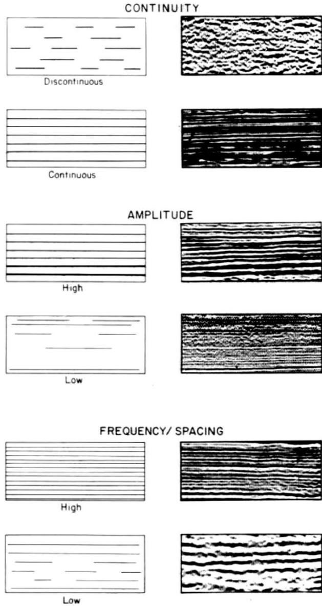
**FIGURE 4.1** Reflection attributes: continuity, amplitude, frequency/spacing.
