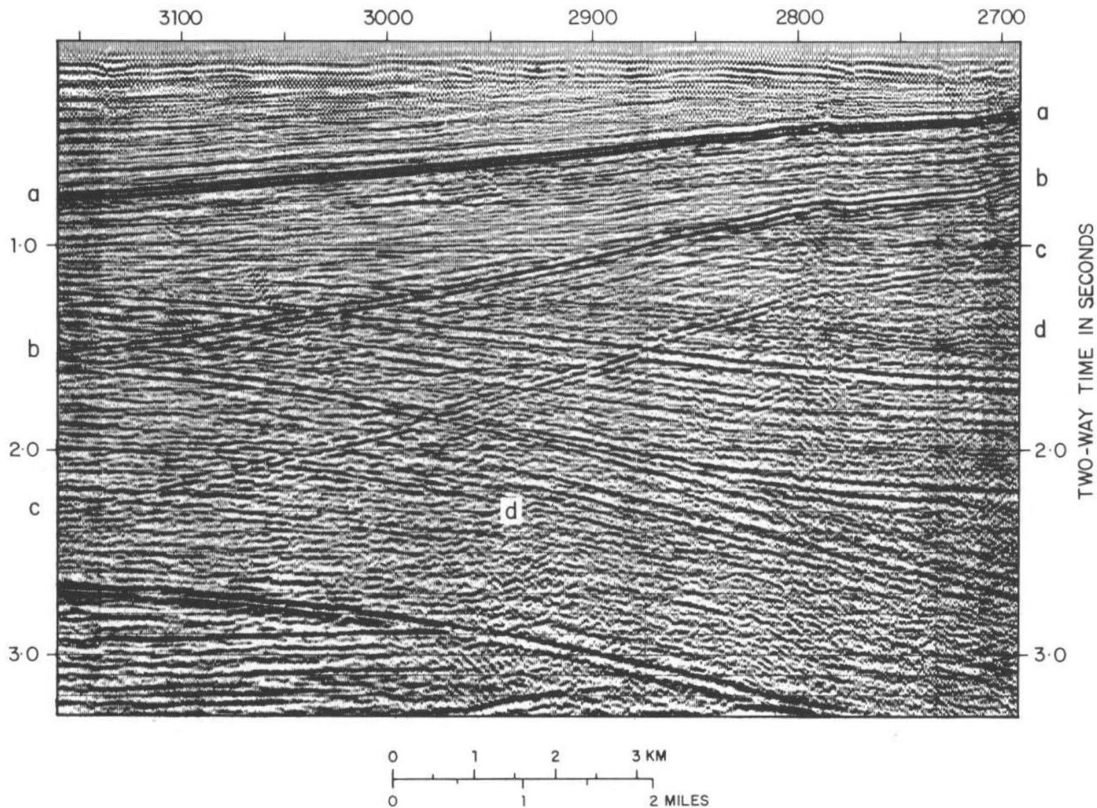
**FIGURE 3.14** Seismic section showing dipping simple multiples from reflection a. Three bounces of the multiples, b, c, and d can be seen. The dip of each successive multiple increases by an amount equal to the dip of the primary reflection a. Courtesy Merlin Profilers Ltd.
