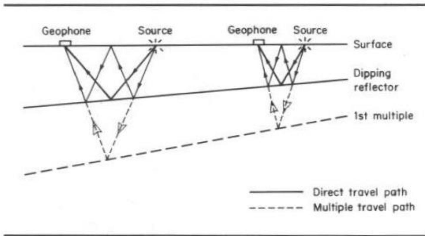
**FIGURE 3.13** Diagram showing how the multiple of a dipping reflector has twice the dip.
