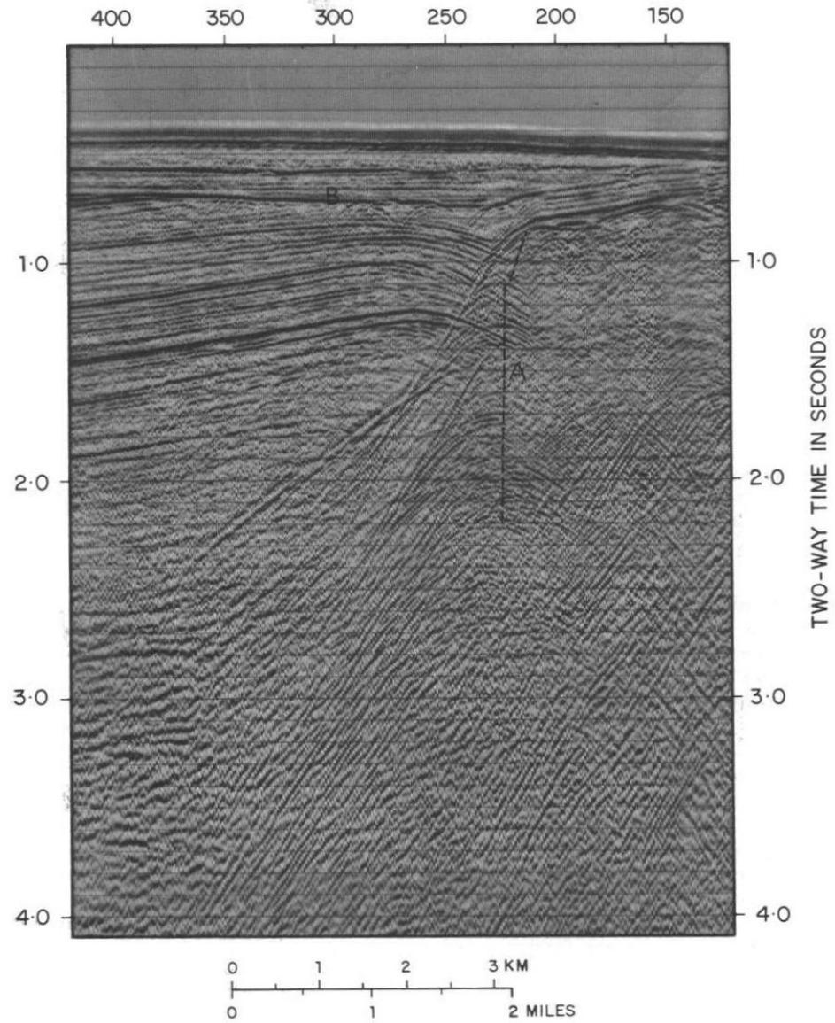
**FIGURE 3.17** Seismic section showing diffractions from a near-vertical fault plane (A). Diffractions can be useful. The fault plane can be located by joining the diffraction apices. Other diffractions are from small faults affecting a flat-lying reflector (B). Courtesy Norsk Hydro.
