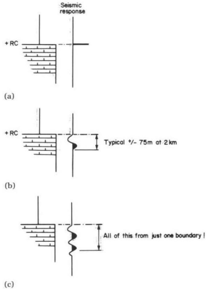
**FIGURE 2.11** *Seismic response at a positive acoustic-impedance boundary. (a) Idealized situation where the seismic response is a spike at each acoustic-impedance boundary. (b) Idealized normal-polarity minimum-phase response of a good seismic system. (c) Response of a poor seismic system that produces a reflection consisting of several cycles from a single boundary.*
