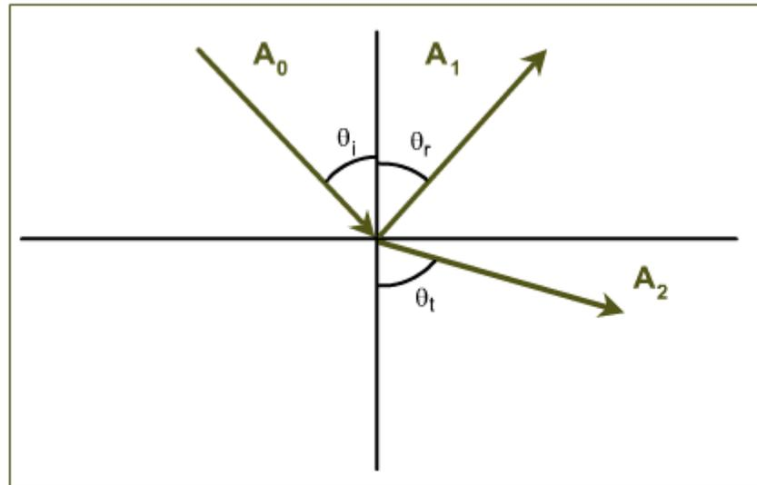
The transmitted wave is refracted according to Snell's law.....
