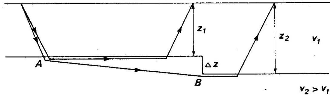
The **throw** on the fault,  $\Delta z$ , can be calculated from the travel time offset,  $\Delta t$
