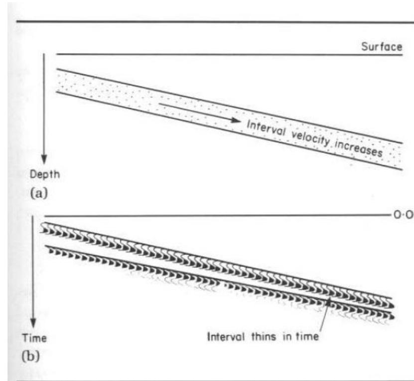
**FIGURE 3.29** *The effect of increasing velocity with depth on the seismic expression of a dipping unit. (a) Geological model of a thick dipping sandstone unit. The sandstone's interval velocity increases with depth due to diagenesis, but its thickness remains constant. (b) Seismic expression: The sandstone unit appears to thin. It takes less time for the seismic signal to travel through the sandstone as its interval velocity increases.*
