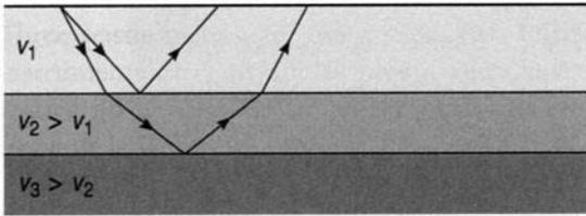
A **thin layer** that does not generate a head wave that is a first arrival
