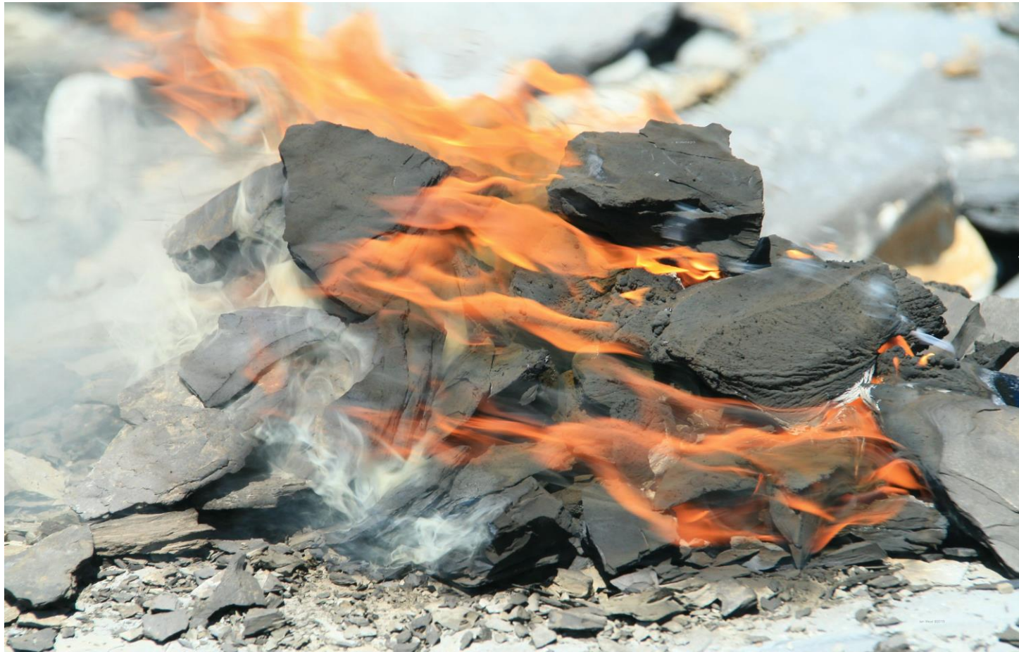
PRODUCTION OF GAS, SULPHUROUS SMOKE AND FLAMES BY BURNING KIMMERIDGE OIL SHALE OR BLACKSTONE - BOTH COMBUSTION AND PYROLYSIS ARE OCCURRING. Some Kimmeridge oil shale was ignited artificially on a Kimmeridge beach and in a slight wind, to examine the mode of burning. Mostly this small fire, once established produced inflammable gas, much of which is burning as detached flames, one or two centimetres or more away from the source, a strongly heated piece of oil shale. On the left of the little fire the heat is affecting ("cooking") the oil shale. There, gas and foul, unhealthy, sulphurous fumes are being produced but have they mostly not ignited; this is a crude example of pyrolysis. Temperatures in burning Kimmeridge oil shale are likely to be round about 500 degrees C. When the shale is partially burnt it becomes yellow and when fully burnt it is red. This takes time and does not happen in a small brief fire. Ian West © 2013.
